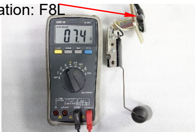
Oil level gauge resistance measurement (full)
