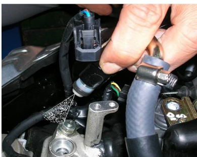
Good injection condition
