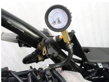
Fuel pressure force measurement disassembly point - fuel injector
