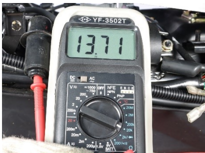
Measurement of the resistance value of the secondary coil terminal
