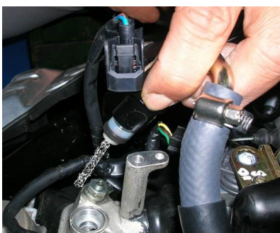
Abnormal jetting condition
