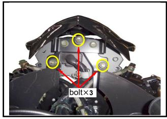
Remove the speed meter stay.
