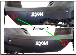
Remove the 2 mounting bolts of the frame.
