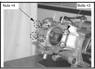
Apply with oil onto the thread of cylinder head bolts and tighten the bolts in diagonally for 2-3 sequences. Do not over tightening the bolts to avoid the cylinder head deformation, noise created or leaking so that effects motorcycle's performance.
