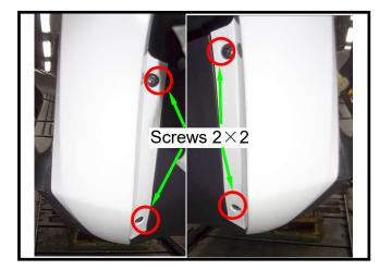
Remove the 2 mounting screws of the floor panel
