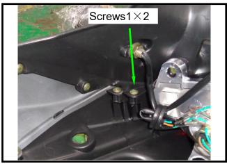
Remove the rear fender.mudguard Remove the rear fender. Remove the rear center cover. Remove the left/right body cover.
