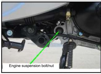
Check if the engine suspension, rear shock absorber bushing, and cushion rubber for damage. Replace them with new ones if so.
