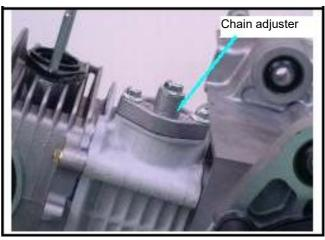
Removed cylinder head side cover.
