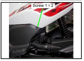
Remove the 4 screws between the center cover and the left/right body cover.
