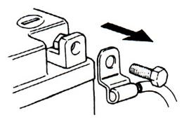
After service completed, make sure all connection points is secured. Battery positive (+) cable should be connected firstly. And the two posts of battery have to be greased after connected the cables.
