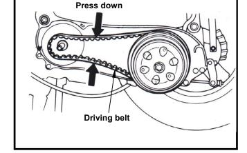
Install driving pulley, washer and nut.
