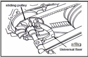
Hold driving pulley with universal fixture, and remove nut and clutch outer.
