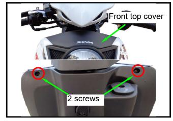
Remove the 2 tapping screws between the front cover and the inner cover.
