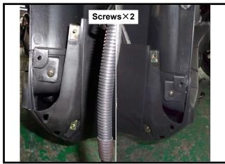
Remove the 2bolts of the frame **Installation**Install the inner cover according to the reverse procedure of removal.
