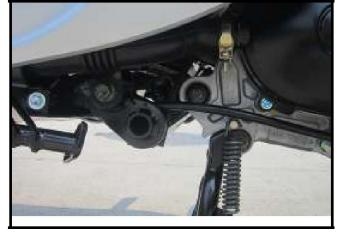
Remove the left side bolt of engine suspension frame.
