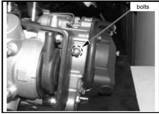
Removed cam chain adjustment bolt. And then removed the chain adjuster (bolts × 2)
