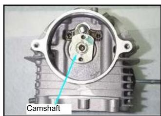
Remove the valve rocker arm shaft.
