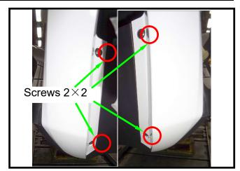
Remove the headlight wire connector and front winker connector then remove the front cover.
