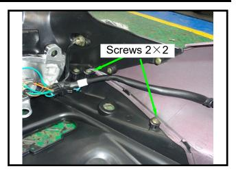
Remove the 6 screws between the rear fender and the left/right body cover.
