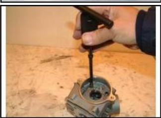
Remove the valve rocker arm.
