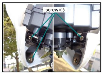
Remove the meter visor stay bolt (2 bolts) between the meter visor stay and the meter
