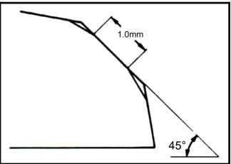
Coat the valve seat surface with red paint. Install the valve through valve guide until the valve contacting with valve seat, slightly press down the valve but do not rotate it so that a seal track will be created on contact surface.
