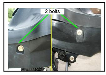
Remove the 4 mounting screws of the floor panel
