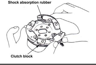
Install the spring snap into groove with pliers.
