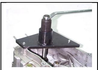
Remove the crankshaft from the right crankcase.
