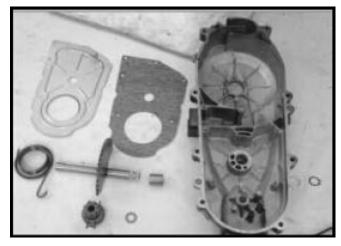
Check if starter shaft, drive gear, bushing, for wear or damage. Replace it with new one if necessary.
