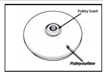
Install siding pulley assembly onto crankshaft.
