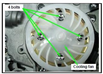
Install the cooling fan shroud. (4 bolts)
