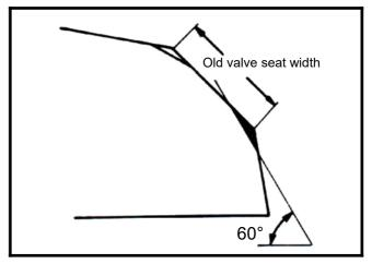
Use 45° cutter to grind the valve seat to specified width.
