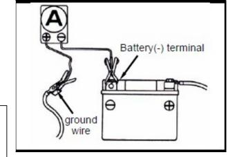
If the leaked current exceeds the specified value, it may indicate a short circuit.
