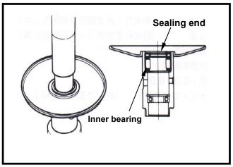
Installation of clutch/driven pulley
