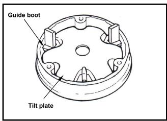
Apply with grease 4~5 g to inside of driving shaft hole, and install driving pulley hub.
