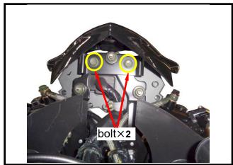
Removed the speed meter stay nut (3 nuts)
