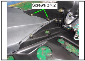
Remove the 2 screws between the rear fender and the rear center cover.
