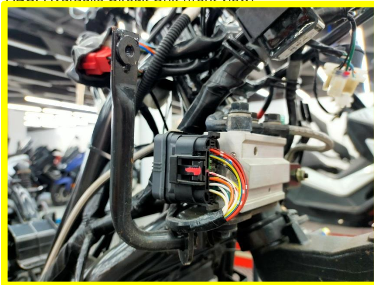
ABS. Hydraulic Circuit Unit (right view)
