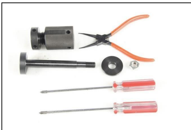
RR. FORK BRG. 6303 INSTALL PULLER
