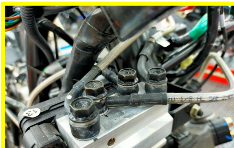
ABS. Hydraulic Circuit Unit (right view)
