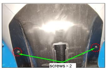
Remove the 4 mounting screws (both side)
