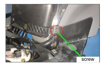
Open the left pillion step Remove the bolt of left body cover
