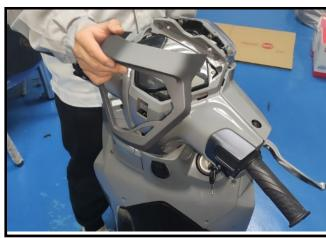
Remove the 6 mounting screws.
