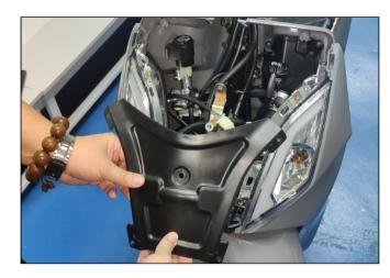
Remove the 2 mounting screws of inner lower cover
