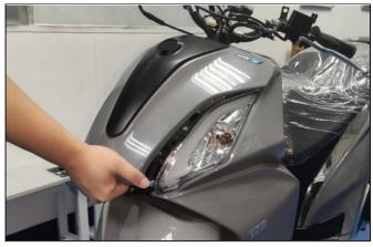
Remove the 4 mounting screws & 2 mounting Bolt.
