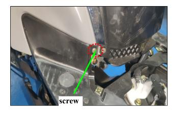
Remove the screw of under cover
