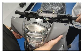
Remove the 3 mounting screw (Pay attention to pulling off the Meter)
