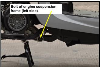
Check if the engine suspension frame bushing and cushion rubber for damage. If so, replace with new ones.
