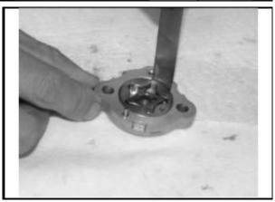
Check clearance between inner and outer rotors.
