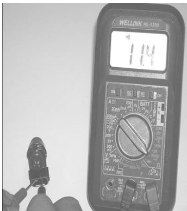
Injector resistance confirmation
