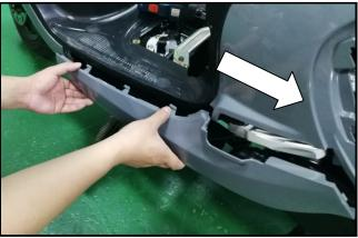
Remove the 9 mounting screws, Remove the mounting bolt.
