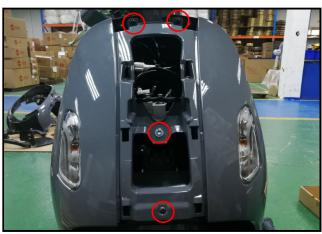
Remove the 2 mounting screws (both side)
