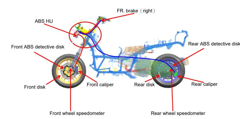
Dual channel ABS front and rear brake system passes HU
