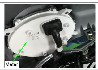
Remove the speedometer cable.
