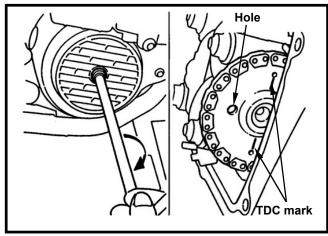
Remove camshaft holder nut and washer.
