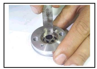
Check clearance between inner and outer rotors.
