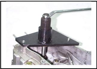
Remove the crankshaft from the right crankcase.
