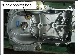
Place the left side of crankcase upward, and then install the crankcase remover/set onto the crankcase.
