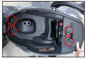
Remove the 3 mounting socket bolts of rear carrier
