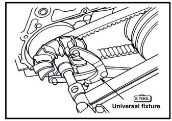
Remove the driving belt from the pulley. Remove sliding pulley set and driving pulley hub from crankshaft.
