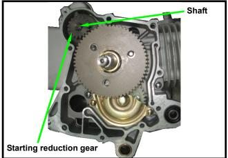
Install the starting clutch outer and starter driven gear.
