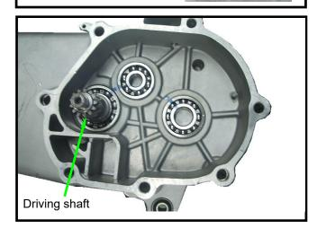
Install a new final driving shaft bearing onto gear box cover.
