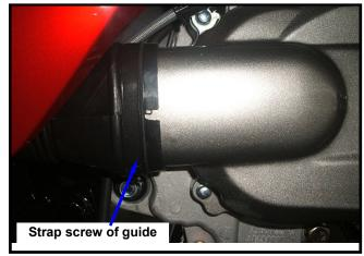
Remove the engine suspension nuts and bolts (engine side), and then remove the engine.
