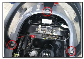
Remove the mounting screw(both side)
