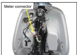
Remove the rear handle cover. Remove the meter mounting screws. Take out the meter.
