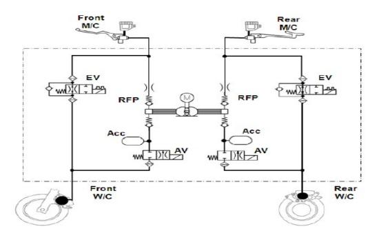
Front wheel oil pressure circuit diagram
