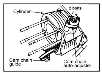
Remove cam chain plate. Remove cylinder.
