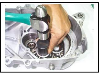
Press out the driving shaft from the crankcase.
