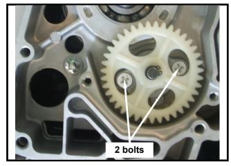
Install oil pump outer cover (2 bolts).
