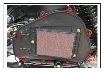
Remove the air cleaner element (3 screws).
