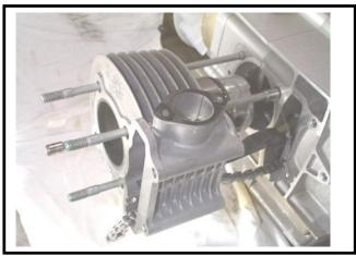
Remove cylinder gasket and lock pins
