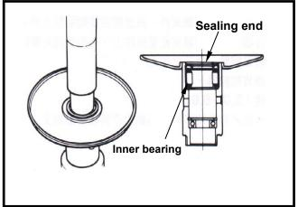
Installation of clutch/driven pulley
