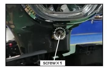
Remove the mounting screws (4 screws) between the front handle cover and the rear handle cover.
