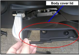
Remove the mounting expansion screws (both side)
