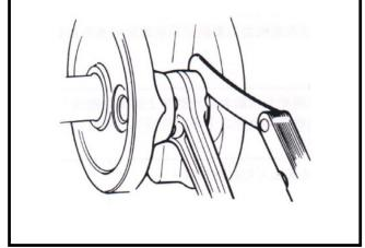
Measure the radical clearance of the big end at the vertical directions.
