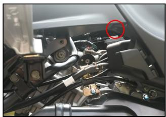
Remove the mounting screw(both side)
