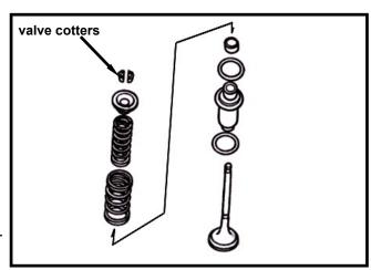
Remove valve stem guide seal.
