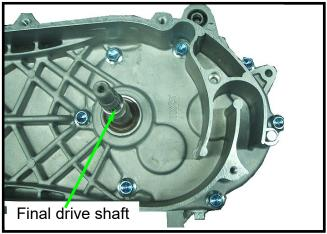
Check bearings on gear box and cover. Rotate each bearing's inner ring with fingers. Check if bearings can be turned in smooth and silent, and also check if bearing outer ring is mounted on gear box & cover tightly. If bearing rotation is uneven, noising, or loose bearing mounted, then replace it. Check oil seal for wear or damage, and replace it if necessary.
