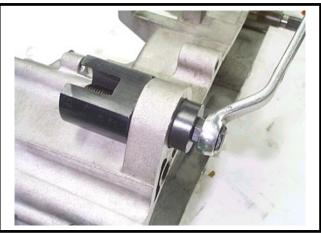
Bolt of engine suspension frame (right side)
