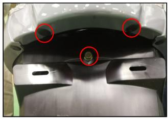
Remove the mounting screw(both side)
