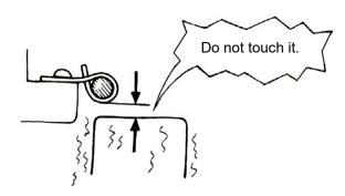
Route wire harness to avoid sharp edges or corners and also avoid the projected ends of bolts and screws.
