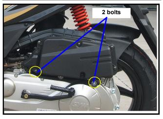
Loosen the air cleaner connecting pipe screw.
