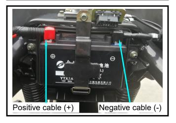
Install the battery in reverse order of removal.
