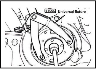
Install the cooling fan. (4 bolts)
