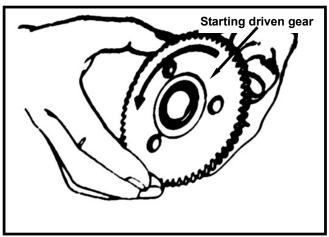
Check the starting driven gear for wear or damage.
