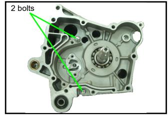
Install the cam chain tensioner.
