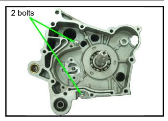
Remove the cam chain tensioner (hex socket bolt) from the left side of crankcase.
