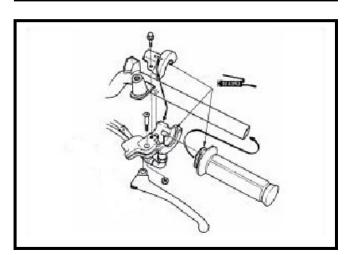
With a wrench to hold the handlebar bolt and then remove the nut.
