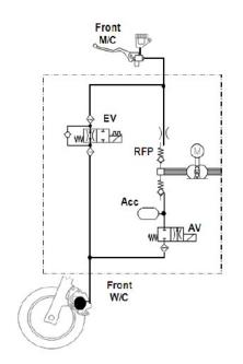
Front wheel oil pressure circuit diagram
