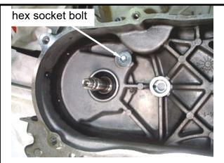
Apply with some grease onto the oil seal lip and then install it onto the left crankcase.
