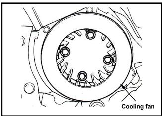
Hold the flywheel with the universal fixture. Remove the 10mm nut on the flywheel.
