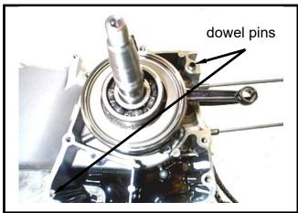
Install the right crankcase and tighten the crankcase bolts (2 bolts).
