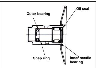
Remove snap ring and then push bearing forward to other side of inner bearing. Place new bearing onto proper position and its sealing end should be forwarded to outside.
