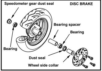
Align the flange part on the speedometer gear with the slot of wheel hub, and then install the brake disc (drum brake) or speedometer gear box.
