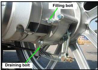
Remove gear oil filling hole bolt and place a measurement cup under the draining plug. Remove the oil draining plug and the pour gear oil into the measurement cup. Measure the gear oil quantity if within standard value.
