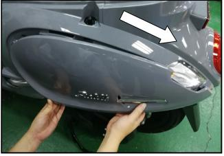
Remove the 2 mounting expansion screws & bolt
