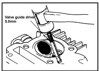
Hold the cylinder head, and then press out old valve guide from combustion chamber side.
