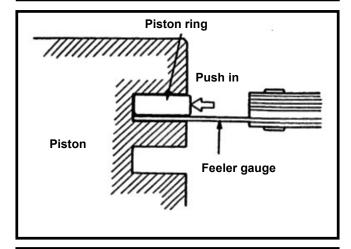
Take out the piston rings and place them respective into cylinder below 20mm of cylinder top. Measure each piston ring gaps.
