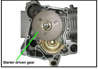
Hold the starting driven gear with the universal fixture.
