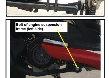
Check if the engine suspension frame bushing and cushion rubber for damage. If so, replace with new ones.
