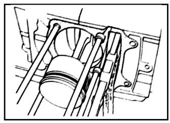
Clean the residues attached onto the matching surfaces of cylinder and crankcase.
