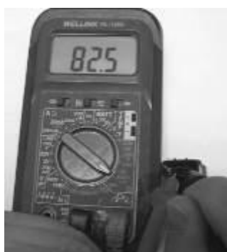
B phase measurement of the resistance value
