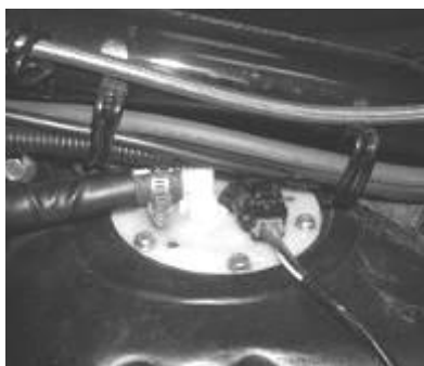
Fuel pressure measurement demolition - fuel pump
