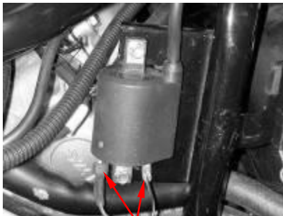
First circuit coil resistance measurement
