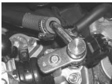
Fuel pressure measurement demolition - injector
