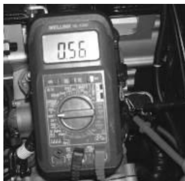
Throttle output signal measurement - full closed
