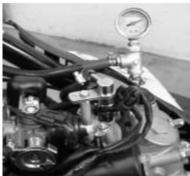
Fuel system pressure measurement
