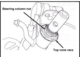
With a plastic hammer to tap the steering column slightly, and then remove the top ball bearing seat.
