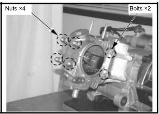
Apply with oil onto the thread of cylinder head bolts and tighten the bolts in diagonally for 2-3 sequences. Do not over tightening the bolts to avoid the cylinder head deformation, noise created or leaking so that effects motorcycle's performance.
