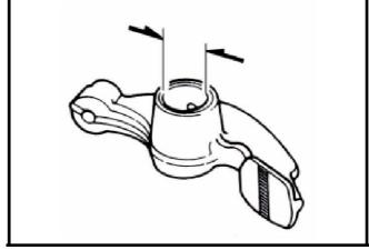
Measure the active O.D. of the valve rocker arm shaft.
