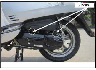
Remove the rear brake cable nut. Remove the rear brake cable. Remove the rear shock absorber lower bolt.
