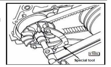
Remove the sliding pulley fixing nut and remove the driving belt from the sliding pulley.
