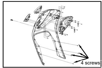
Remove the  $2\times 2$  mounting bolts between the under cover and the frame.
