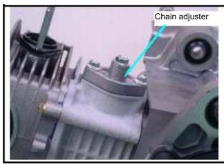
Removed cylinder head side cover.
