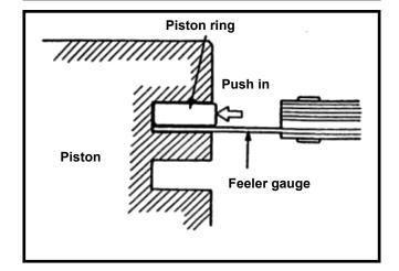
Take out the piston rings and place them respective into cylinder below 20mm of cylinder top. Measure each piston ring gaps.
