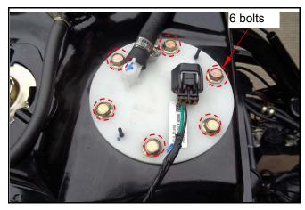
Remove the fuel pump and fuel unit.
