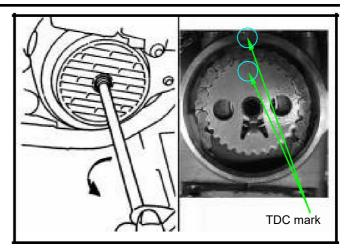
Remove camshaft sprocket bolt(bolt × 2). Remove the cam sprocket and cam chain.
