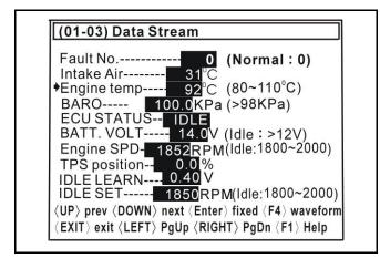
Press <F1> button to enter description page. Press any key to get back to Data Stream page. Engine temp-----This data can be used for observing the engine been warm-ready or not. Some ECU control items need impleted in egine warm-ready status.
