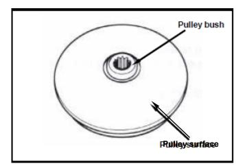
Install siding pulley assembly onto crankshaft.
