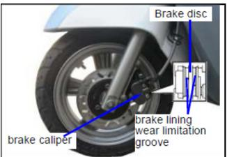
Park the motorcycle on a flat ground and check its brake fluid level.
