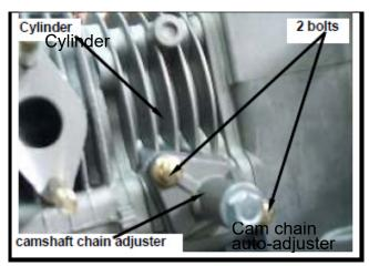
Remove cam chain plate. Remove cylinder.
