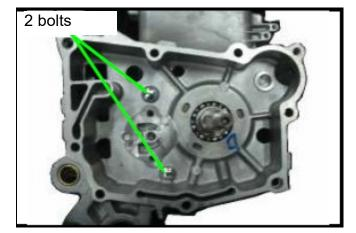
Install the cam chain tensioner.
