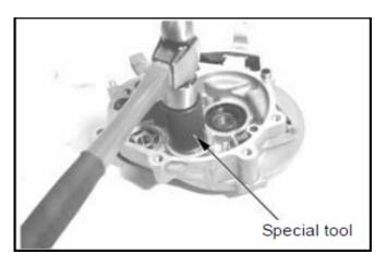
Press out the driving shaft from the crankcase.
