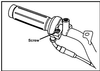
Remove the rear brake lever nut and screw, then take out the rear brake cable.
