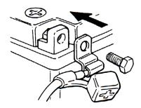
Make sure that the battery post caps are located in properly after the battery posts had been serviced.
