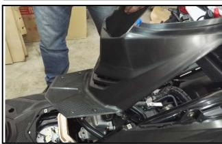
Disconnect the fuel pump couplers. Disconnect the fuel unit couplers Remove the fuel pipes.
