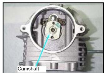
Remove the valve rocker arm shaft.
