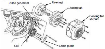
Drain out the engine oil. Remove the exhaust muffler. (2 bolts, 2 nuts) Remove the fan shroud. (4 bolts)
