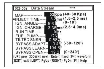
Press <F1> button to enter description page. Press any key to get back to Data Stream page. INJECT TIME-----ECU set the injetter ON time interval
