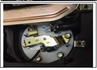
Remove the fuel pump lock bolts.
