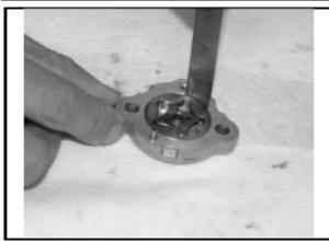
Check clearance between inner and outer rotors.
