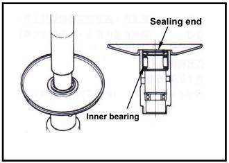
Installation of clutch/driven pulley
