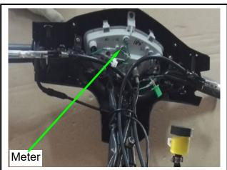
Remove the speedometer cable.
