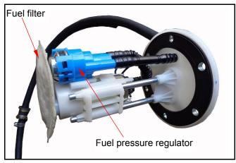
Remove the fuel unit. Check the oil seal of fuel unit for any damage or deformation.
