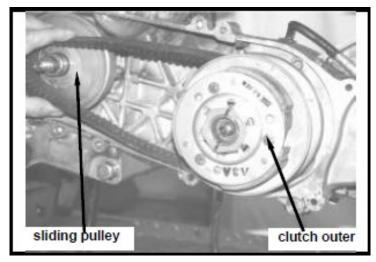
Install the clutch with universal fixture, and then tighten nut to specified torque value. Torque value: 3.5~4.5 kgf-m
