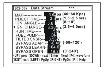
Press <F1> button to enter description page. Press any key to get back to Data Stream page. IGN. CHARGE-----ECU set the ignition transistor ON ti
