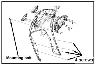
Remove the 2 mounting screws and between the front cover and inner box.
