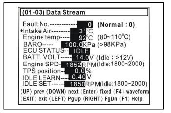
Press <F1> button to enter description page. Press any key to get back to Data Stream page. Intake Air----Measure the intake air temperature to c onvey to ECU, then the ECU calculate o ut proper compensation and controllin g amount of injetted fuel.
