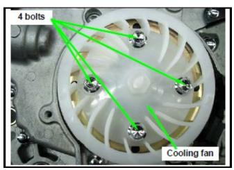
Install the cooling fan shroud. (4 bolts)
