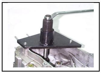
Remove the crankshaft from the right crankcase.
