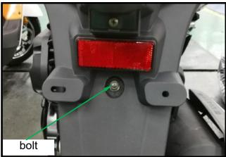
Remove the 2 mounting screws of body cover.
