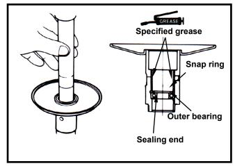
Install a new inner bearing.
