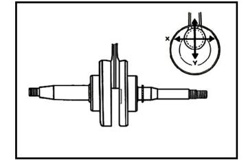
Place the crankshaft onto a V-block and measure run-out of the crankshaft with dial gauge.
