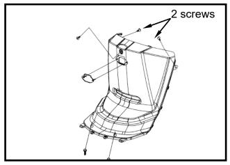
Remove the mounting bolt of rear fender.
