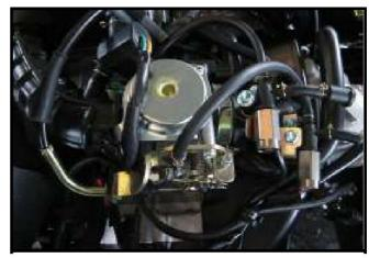
Remove the exhaust muffler (Bolts × 2, Nuts × 2).
