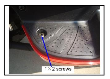
Remove the 4 mounting screws between the front cover .
