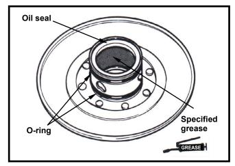
Install sliding pulley onto driven pulley. Install guide pin and guide pin roller.
