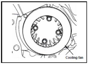
Hold the flywheel with the universal fixture. Remove the 10mm nut on the flywheel.
