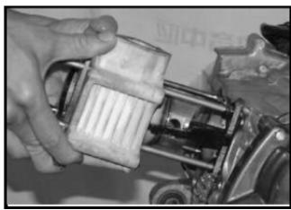
Remove cylinder gasket and lock pins
