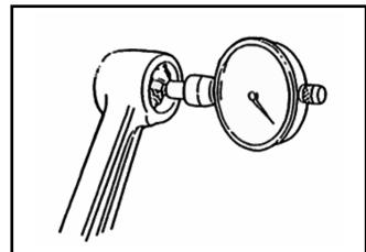
Measure the inner diameter of piston pin hole.
