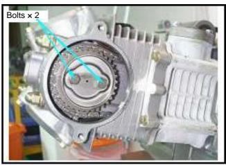
Removed the bolts of the left side of the cylinder head between cylinder head and cylinder(bolt × 2).
