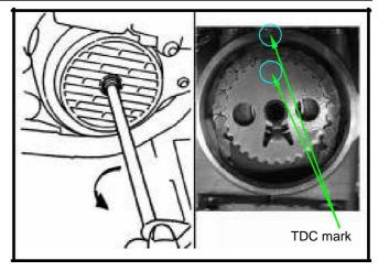
Remove camshaft sprocket bolt(bolt × 2). Remove the cam sprocket and cam chain.
