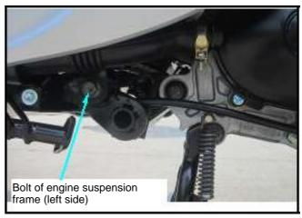
Check if the engine suspension frame bushing and cushion rubber for damage. If so, replace with new ones.
