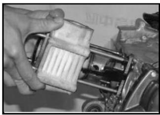
Remove cylinder gasket and lock pins
