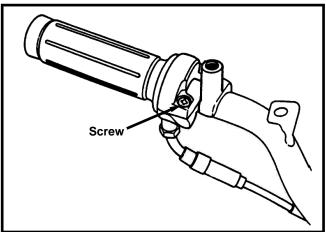
Remove the rear brake lever nut and screw. then take out the rear brake cable. Remove the brake lever seat bolt, and then remove the seat.
