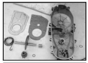
Check if starter shaft, drive gear, bushing, for wear or damage. Replace it with new one if necessary.
