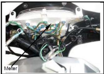
Remove the speedometer cable.
