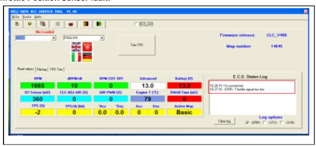
When throttle position sensor problem happened, the software shows that throttle signal too low(show as the above picture)
