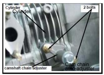
Remove cam chain plate. Remove cylinder.
