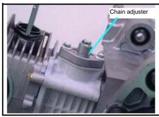
Removed cylinder head side cover.
