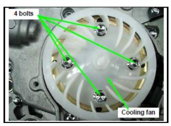
Install the cooling fan shroud. (4 bolts)
