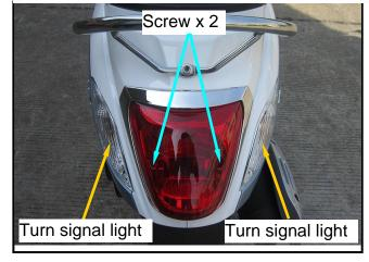
Replace the bulbs of the tail light, brake light (12V 5W/21W)
