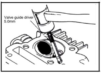
Hold the cylinder head, and then press out old valve guide from combustion chamber side.
