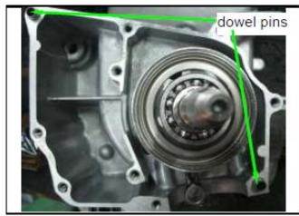
Install the right crankcase and tighten the crankcase bolts (1 bolts).
