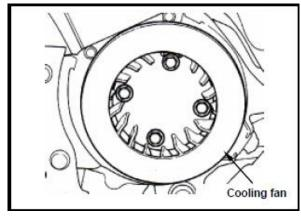
Hold the flywheel with the universal fixture. Remove the 10mm nut on the flywheel. **Special Service Tools: Universal Fixture**
