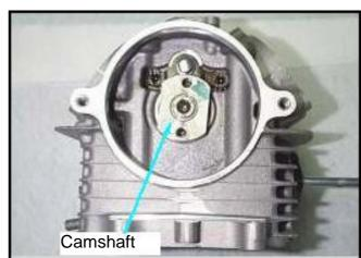
Remove the valve rocker arm shaft.
