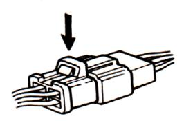
Do not pull the wires as removing a connector or wires. Hold the connector body.
