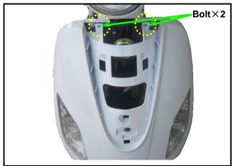
Remove the front under cover 4 mounting screws between the front under cover and the frame .
