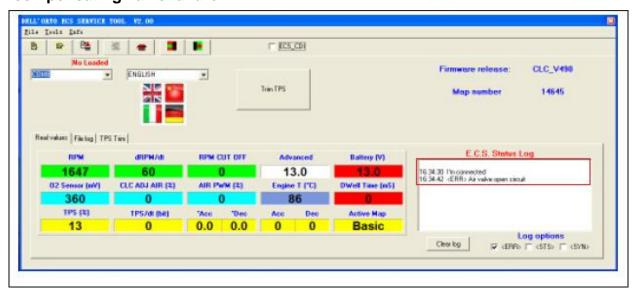
When solenoid valve problem happened, the software shows that air valve open circuit (show as the above picture)
