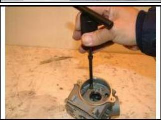
Remove the valve rocker arm.
