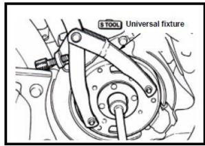
Remove the flywheel with the flywheel puller.
