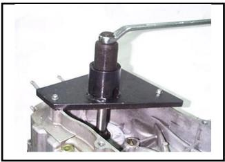
Remove the crankshaft from the right crankcase.
