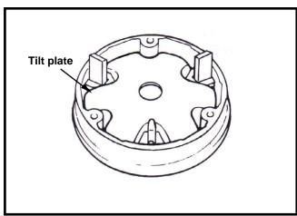
Remove weight rollers from sliding pulley.
