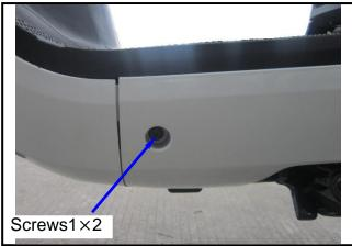
Remove the left/right side 2 mounting bolts in the rear of the side cover.
