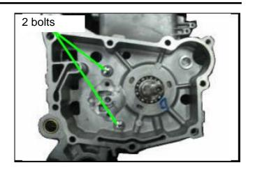
Remove the cam chain tensioner (hex socket bolt) from the left side of crankcase.
