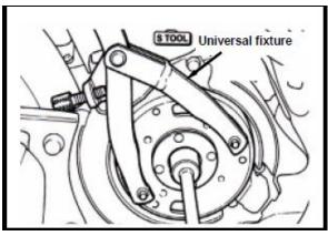
Install the cooling fan. (4 bolts)
