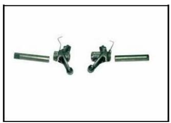
Use the special tool of compress valve springs. Remove valve spring removed location pin.
