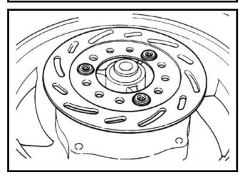
Remove the left axle ring and dust seal. Remove the dust seal on the right side of speedometer gear.
