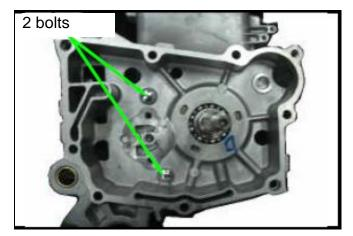
Install the cam chain tensioner.
