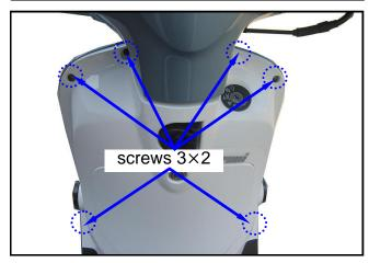
Remove the hook screw bolt from the front inner box.
