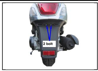
Remove the 2 mounting screws between the body cover and the frame.
