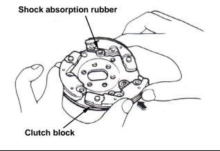
Install the spring snap into groove with pliers.
