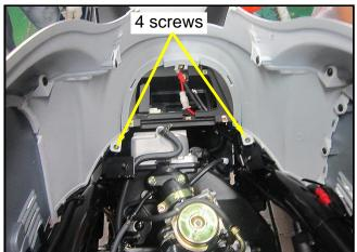
Remove the rear fender. Remove the left/right body cover.
