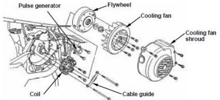
Drain out the engine oil. Remove the exhaust muffler. (2 bolts, 2 nuts) Remove the fan shroud. (4 bolts)
