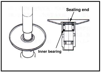
Installation of clutch/driven pulley
