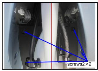
Remove the 2 mounting screws between the front cover and the left/right side cover.
