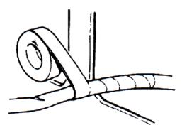
Secure the rubber boot firmly as applying it on wire harness.
