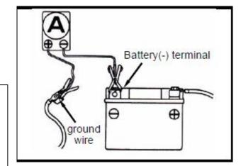
If the leaked current exceeds the specified value, it may indicate a short circuit.
