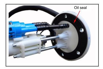
Check if the fuel filter is contaminated or clogged. Replace it with new one if necessary.
