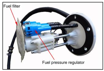
Remove the fuel unit. Check the oil seal of fuel unit for any damage or deformation.
