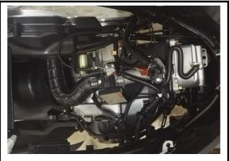
Remove the fuel tube. Remove cylinder head TEMP sensor connector.
