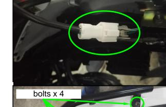
Remove the 4 mounting bolts of rear carrier
