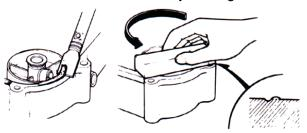
The ends of rubber hoses (for fuel, vacuum, or coolant) should be pushed as far as they can go to their connections so that there is enough room below the enlarged ends for tightening the clamps.
