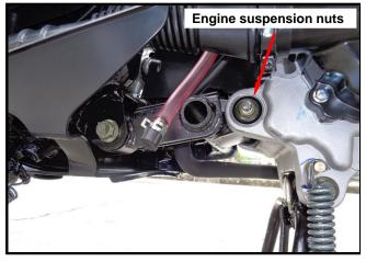
Check if the engine suspension, rear shock absorber bushing, and cushion rubber for damage. Replace them with new ones if so.
