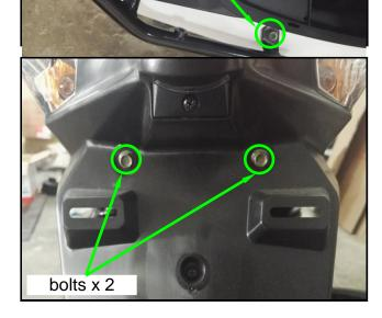
Remove the 2 mounting bolts of rear fender
