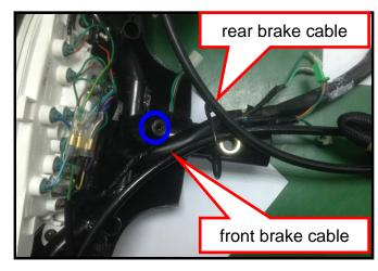
Install the front brake cable to left side handle lever.
