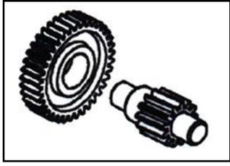
Check if the final driving shaft and gear are burn, wear or damage.
