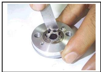
Check clearance between rotor side face and pump body.
