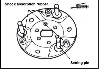
Apply with grease onto setting pins. But, the clutch block should not be greased. If so, replace it.
