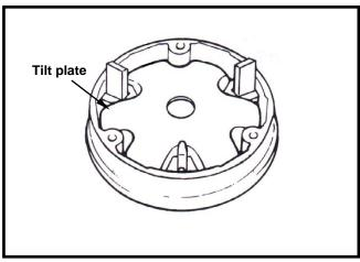
Remove weight rollers from sliding pulley.
