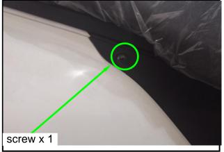
Remove the 2 mounting screws between the body cover and center cover.
