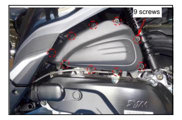
Remove the air cleaner element (3 screws).
