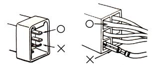
Insert the connector completely. If there are two lockers on two connector sides, make sure the lockers are locked in properly. Check if any wire loose.
