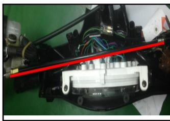
Turn back the front brake cable end bolt by slowly, make the another side cable end can touch the brake lever setting.
