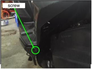
Remove the mounting screw front of right side cover.
