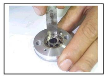
Check clearance between inner and outer rotors.
