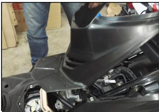
Remove the mounting screw front of left side cover.
