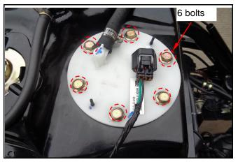
Remove the fuel pump and fuel unit.
