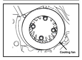
Install the cooling fan shroud. (4 bolts)
