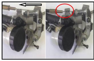
Install the front brake cable and lock the brake cable end nut
