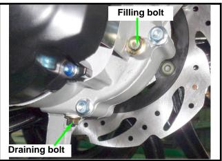
Remove gear oil filling hole bolt and place a measurement cup under the draining plug. Remove the oil draining plug and the pour gear oil into the measurement cup. Measure the gear oil quantity if within standard value.
