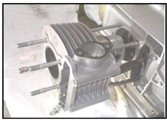
Remove cylinder gasket and lock pins
