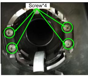
Open the fuel tank cap and remove the 4 mounting screw of fuel tank
