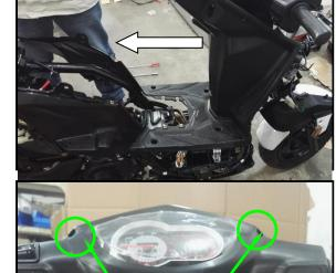
Remove the mounting screw of front handle Cover.
