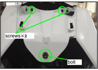
Remove the mounting screw of left side inner fender.
