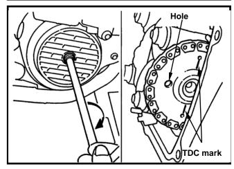
Remove camshaft holder nut and washer.
