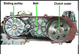
Install the clutch with universal fixture, and then tighten nut to specified torque value.
