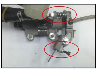
Install the rear brake cable install the cable inside the CBS gap.
