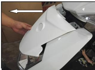
Remove the 2 mounting screws and 1 bolt
