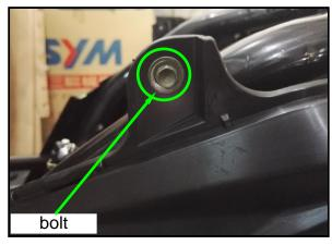
Remove the mounting bolt upper of Floor panel left side.
