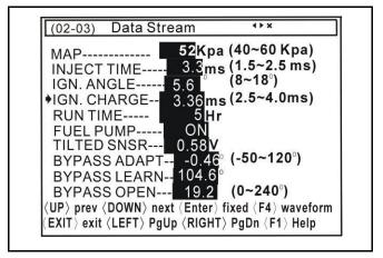
Press <F1> button to enter description page. Press any key to get back to Data Stream page. IGN. CHARGE------ECU set the ignition transistor ON time interval (Ignition energy).
