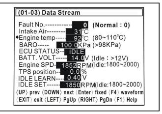
Press <F1> button to enter description page. Press any key to get back to Data Stream page. Engine temp-----This data can be used for observing the engine been warm-ready or not. Some ECU control items need impleted in egine warm-ready status.
