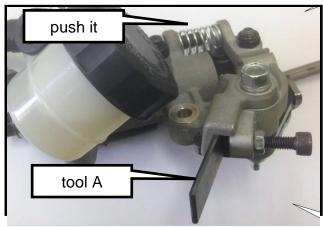
Install the front brake cable. inside the cable end to swing arm.
