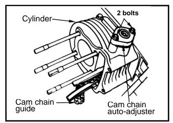
Remove cam chain plate. Remove cylinder.
