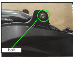
Remove the mounting screw of inner cover
