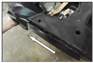
Remove the mounting screw front of Floor panel left side.
