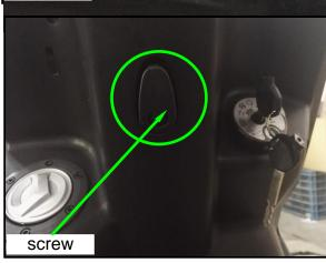
Remove the mounting screw of main switch
