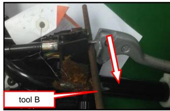
Be careful the handle stay when insert the front brake cable and rear brake cable.
