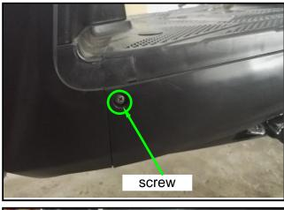
Remove the mounting screw back of left side cover.
