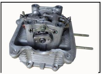
After removed valve cotters, release the compressor and then take out spring retainer, valve spring and valves.
