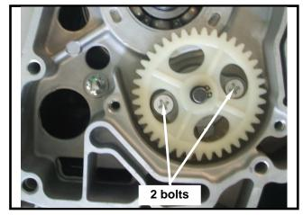
Install oil pump outer cover (2 bolts).
