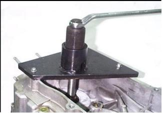
Remove the crankshaft from the right crankcase.
