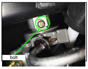
Remove the 2 mounting screw of front inner Fender.
