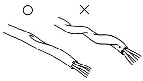
Wire harnesses routed along the handlebar should not be pulled too tight or have excessive slack, be rubbed against or interfere with adjacent or surrounding parts in all steering positions.
