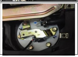
Remove the fuel pump lock bolts.
