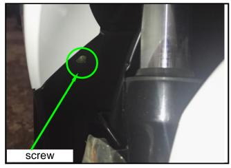
Remove the 8 mounting screws of inner cover.
