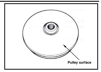
Install siding pulley assembly onto crankshaft.
