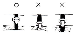
Wire band and wire harness have to be clamped secured properly.
