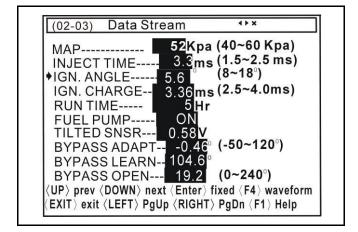
Press <F1> button to enter description page. Press any key to get back to Data Stream page. IGN. ANGLE-----ECU set the engine ignition angle (Ign ition timing).
