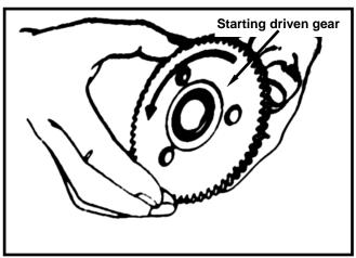
Check the starting driven gear for wear or damage.
