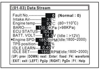
Press <F1> button to enter description page. Press any key to get back to Data Stream page. Engine SPD-----Utilize the crankshaft position senso r with the gear teeth to calculate ou t the engine RPM count.
