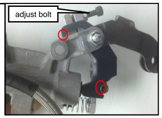
Add brake fluid and exclude air in brake fluid, make the pads clearance more than disk thickness.
