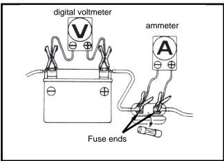
Turn on the headlight to high beam and start the engine.
