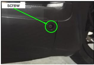
Remove the mounting screw back of right side cover.
