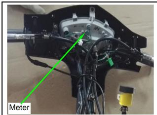
Remove the speedometer cable.
