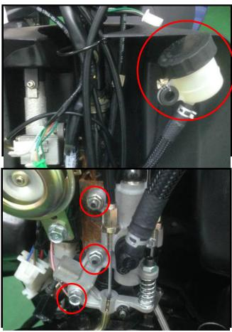
Install the front brake hose and the rear brake cable.
