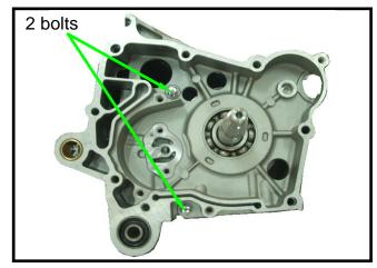
Install the cam chain tensioner.
