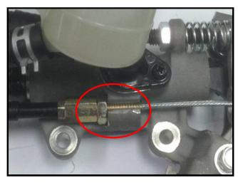
Lock the rear brake wire nut in torque
