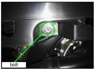
Remove the mounting bolt upper of Floor panel right side.
