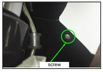
Remove the mounting screw of right side inner fender.
