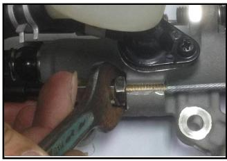
Install the front brake cable to right side handle lever.
