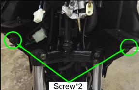
Remove the 2 mounting screws of Under Spolier
