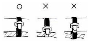
Wire band and wire harness have to be clamped secured properly.
