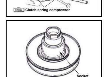
Remove oil seal from driven pulley. Remove guide pin, guide pin roller, and sliding pulley, and then remove O-ring & oil seal seat from sliding pulley.
