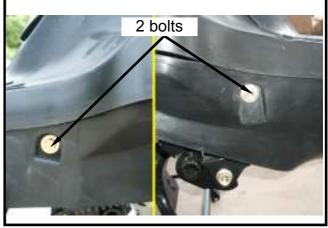
Remove the 2 mounting screws between the front under cover and the floor panel.
