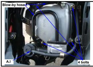
Remove the 2 cylinder head mounting bolts from cylinder head left side cover.
