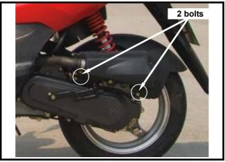
Remove the rear brake cable nut. Remove the rear brake cable. Remove the rear shock absorber lower bolt.
