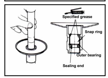
Install a new inner bearing.
