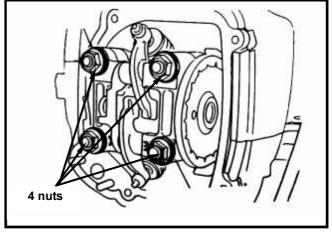
Remove the camshaft holder and rocker arm set.
