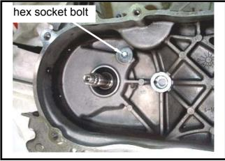
Apply with some grease onto the oil seal lip and then install it onto the left crankcase.
