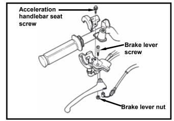
Remove the 2 bolts of the brake master cylinder, and then take out the master cylinder and the split ring.
