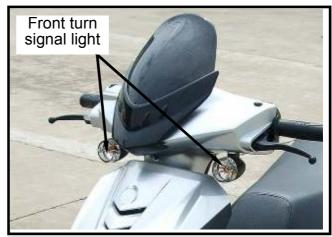
Pull out the bulb and replace it with new one. (12V 5W)
