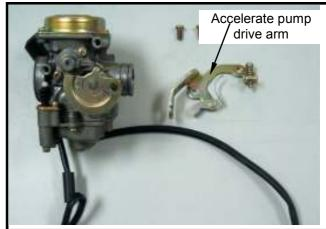
Remove 3 mounting screws and remove the float chamber cover.
