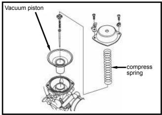
Remove fuel needle seat, spring, and injector needle.
