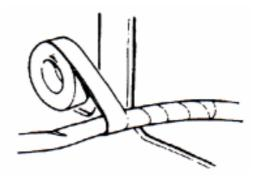
• Secure the rubber boot firmly as applying it on wire harness.
