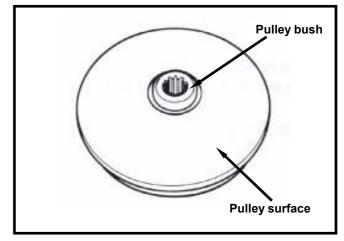
Install siding pulley assembly onto crankshaft.
