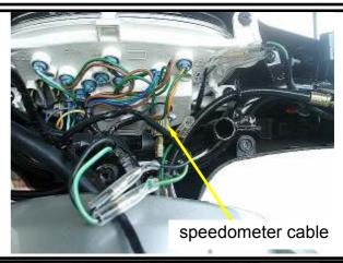
Remove the front cover. Remove the power connector of the meter.
