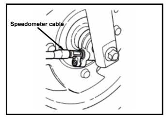
Remove the wheel axle nut and pull out the axle. Then, remove the front wheel.
