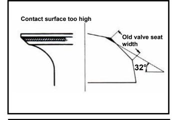
If the contact surface too high, grind the valve seat with 32° cutter.
