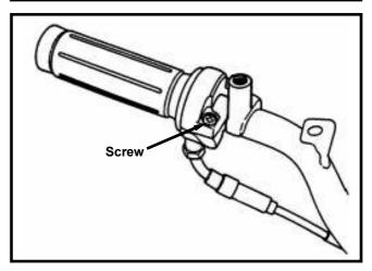
Remove the rear brake lever nut and screw, then take out the rear brake cable. Remove the brake lever seat bolt, and then remove the seat.
