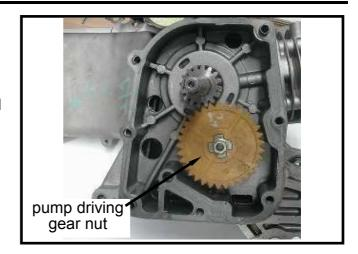
Remove oil pump body bolts (3 bolts).
