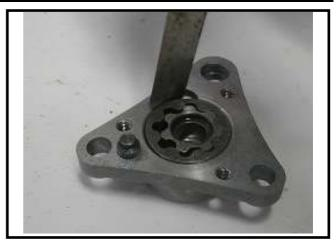
Check clearance between inner and outer rotors.
