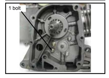
Install the cam chain tensioner.
