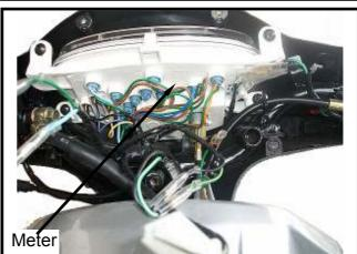
Remove the speedometer cable.
