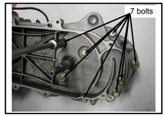
Remove countershaft and gear. Remove final driving gear and shaft.
