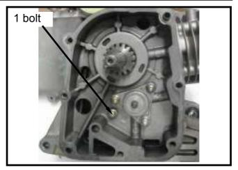
Remove the cam chain tensioner (hex socket bolt) from the left side of crankcase.
