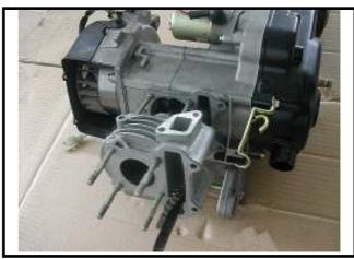
Remove cylinder gasket and lock pins
