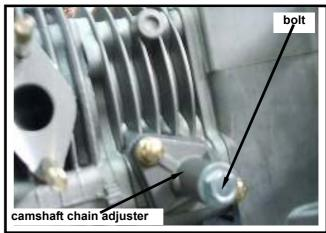
Turn the flywheel in counter clockwise motion with T type wrench until the "T" mark on flywheel aligned with the mark on the crankcase so that the hole on the camshaft sprocket is forward up and piston is at TDC position.
