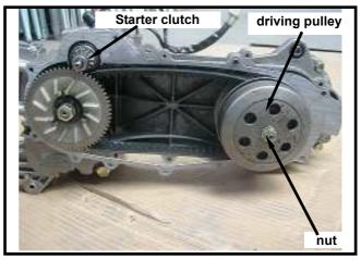
Remove the sliding pulley fixing nut and remove the driving belt from the sliding pulley.
