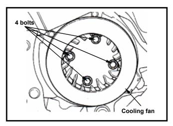
Install the cooling fan shroud. (4 bolts)
