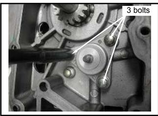
Install the oil pump driving gear nut.
