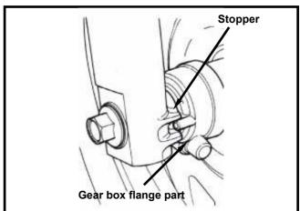
Install the front wheel axle from right shock absorber side.
