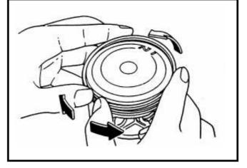
Install the piston rings and then measure clearance between piston ring and its grooves.
