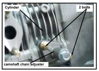
Remove cam chain plate. Remove cylinder.
