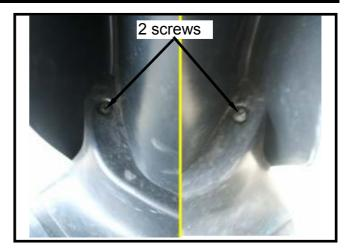
Remove the 4 mounting screws between the front under cover and the inner box B.
