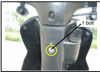
Remove the front cover. Remove the screw on the main switch. Remove the main switch cover.
