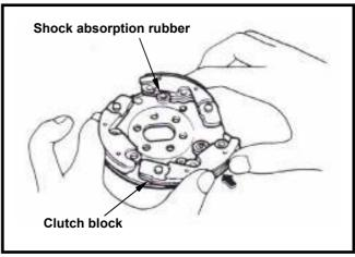
Install the spring snap into groove with pliers.
