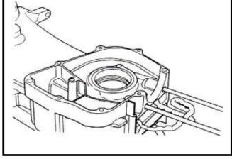
Install crankshaft into the left crankcase and then install two dowel pins and new crankcase gasket.
