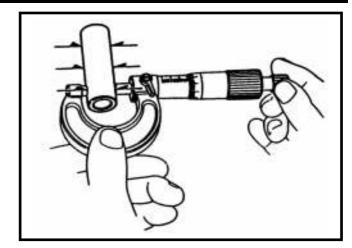
Measure the inner diameter of connecting rod small end.
