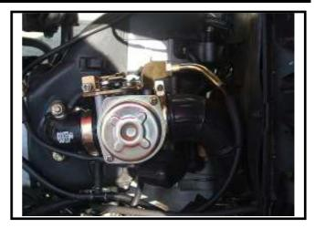
Remove the exhaust muffler (Bolts × 2, Nuts × 2).
