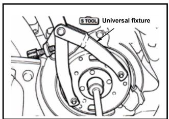
Remove the flywheel with the flywheel puller. Special service tools:
