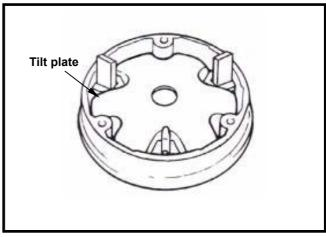
Remove weight rollers from sliding pulley.
