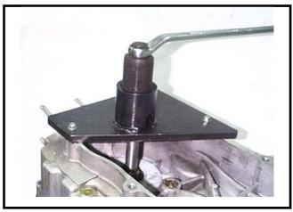
Remove the crankshaft from the right crankcase.
