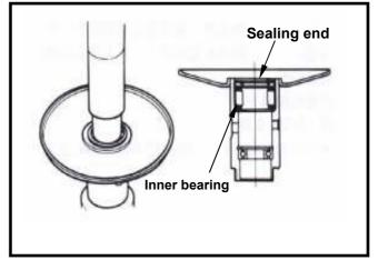
Installation of clutch/driven pulley
