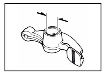
Measure the active O.D. of the valve rocker arm shaft and valve rocker arm.
