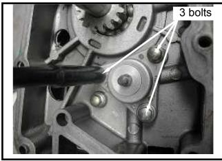
Remove the oil pump pin. Remove the oil pump.
