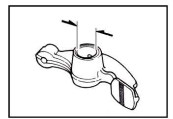
Measure the active O.D. of the valve rocker arm shaft.
