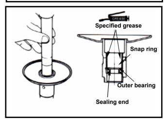
Install a new inner bearing.
