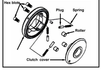
Measure the OD of the starting clutch cover. **Service Limit:**
