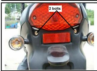
Remove the 2 mounting screws between the body cover and the floor panel.
