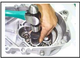
Press out the driving shaft from the gear box. Remove oil seal from the gear box. Remove the driving shaft bearing from the gear box cover with the inner type bearing puller.
