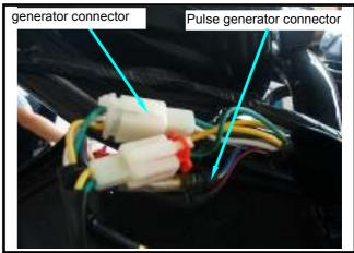
Remove the 6 bolts for the pulse generator, the A.C. generator coil and cable guide. Then, remove the A.C. generator assembly.
