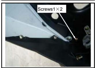
Remove the rear fender. Remove the rear center cover. Remove the left/right body cover.
