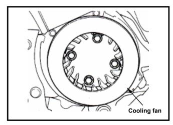
Install the cooling fan shroud. (4 bolts)
