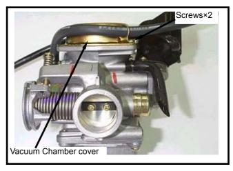
Remove compress spring and vacuum piston.
