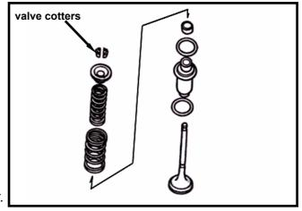
Remove valve stem guide seal. Clean carbon deposits in combustion chamber. Clean residues and foreign materials on cylinder head matching surface.
