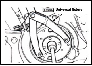
Install the cooling fan. (4 bolts)
