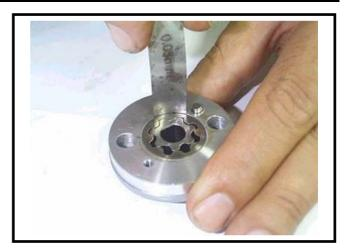
Check clearance between inner and outer rotors.
