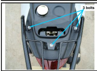
Remove the 2 mounting bolts of the rear fender.
