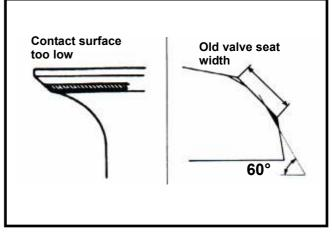
After the valve seat grinded, coat valve seat surface with emery and then slightly press the grinded surface.
