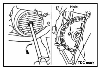
Remove camshaft holder nut and washer.
