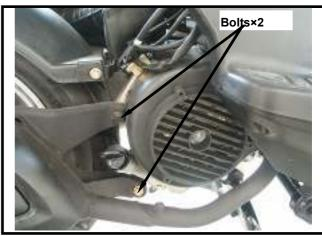
Remove the rear wheel (Nut  $\times$  1).
