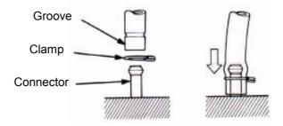
Rubber and plastic boots should be properly reinstalled to the original correct positions as designed.
