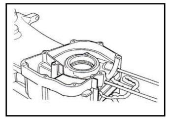
Install crankshaft into the left crankcase and then install two dowel pins and new crankcase gasket.
