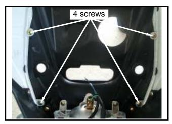
Remove the 4 screws between the rear fender and the left/right body cover.
