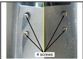
Remove the front inner box A and the front inner box B.
