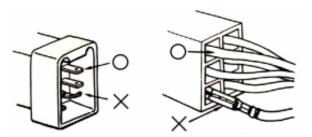
Insert the connector completely. If there are two lockers on two connector sides, make sure the lockers are locked in properly. Check if any wire loose.
