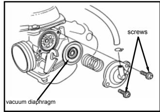
Remove the spring and vacuum diaphragm. Check if the vacuum diaphragm for deterioration or crack.
