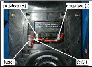
Install the battery in reverse order of removal.
