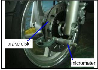
Remove the brake disk from wheel. Check the disk for deformation and bend.
