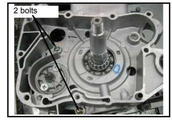
Install the cam chain tensioner.
