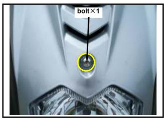
Remove the headlight wire connector and then remove the front cover.
