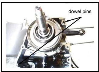
Install the right crankcase and tighten the crankcase bolts (2 bolts).
