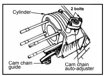
Remove cam chain plate. Remove cylinder.
