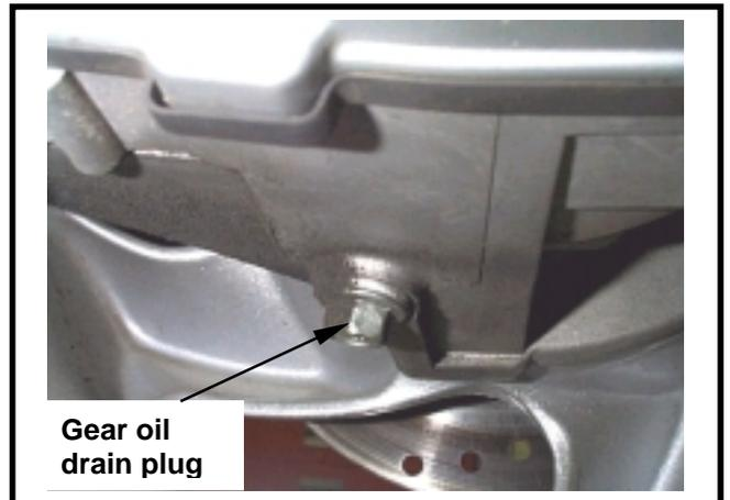
Gear oil drain plug
