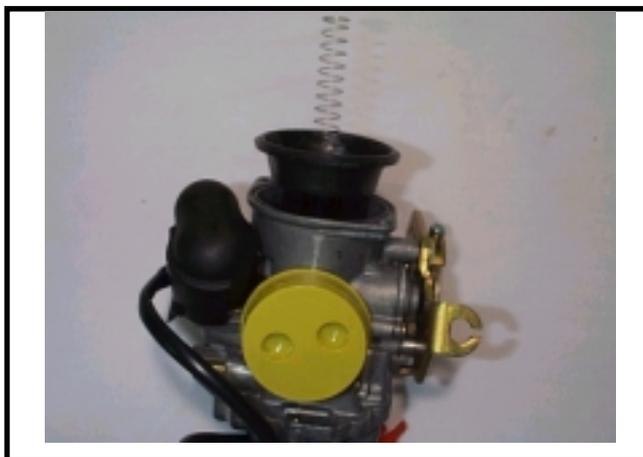
Check if the vacuum piston for wear out, crack or other damage.
