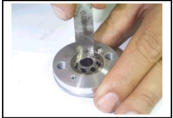
Check clearance between inner and outer rotors.
