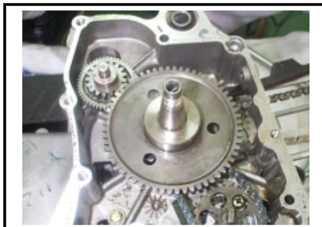
Remove mounting plate, starter reduction gear, and the shaft.
