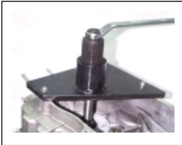
Install the left crank case bearing
