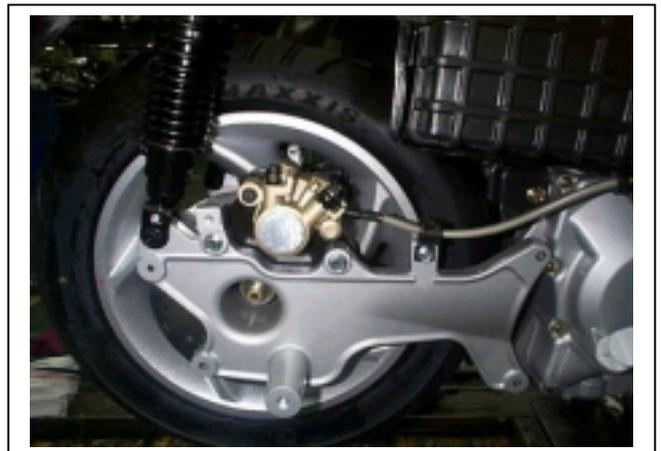
Remove an upper bolt from the shock absorber (bolt x 1).
