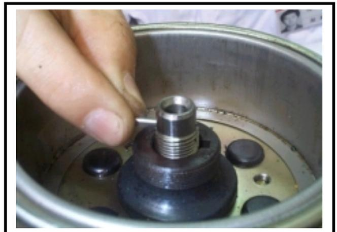
Hold flywheel with flywheel holder, and then remove flywheel nut.
