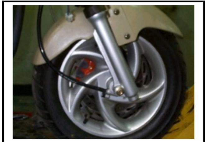
Tighten the nut for the wheel axle.
