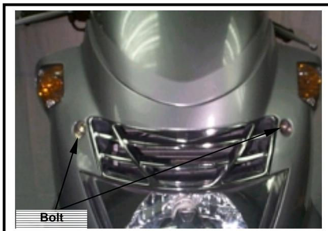
Loosen four screws on the lower part of the front cover.
