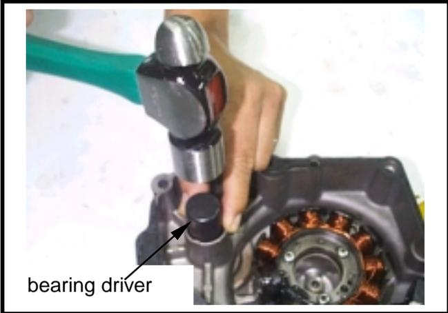
Install the new inner seal onto the right crankcase.
