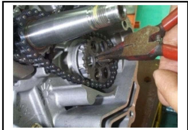
Install starting gear and generator.
