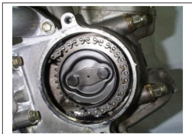
Remove the 2 cylinder head mounting bolts from cylinder head side cover, and then remove 4 nuts and washers from cylinder head upper side.
