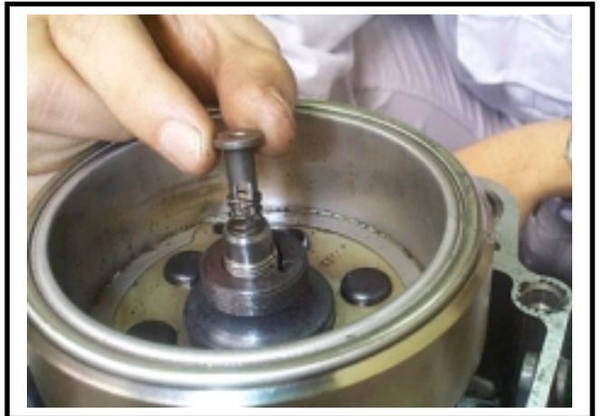
Remove the pin from crankshaft.
