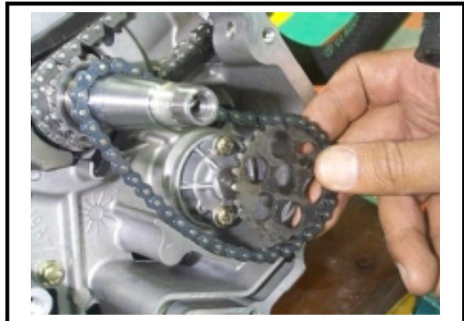
Remove 2 bolts on the oil pump, and then remove oil pump.
