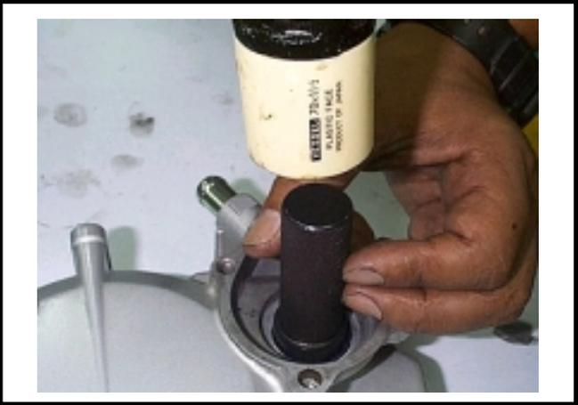
Apply a coat of sealant to the mating surfaces of the right crankcase before installing the new oil seal.
