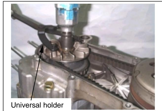
Hold generator flywheel with universal holder, and then remove drive face nut.
