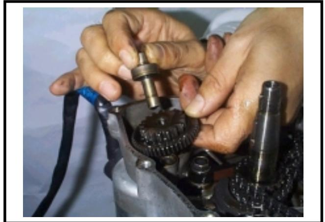
Install one way clutch onto starting clutch gear. Hold flywheel and rotate starting clutch gear. The starting clutch gear should be rotated in C.C.W direction freely, but not C.W direction. (View as shown in this figure.)
