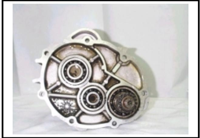
Install the driving shaft onto gear box cover and then place it to proper position.
