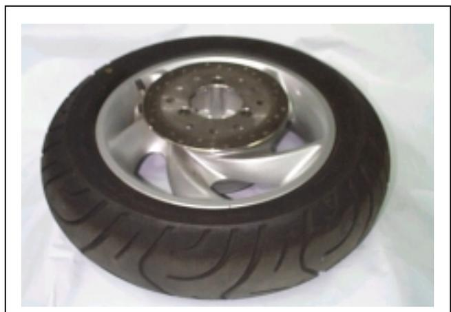
Check any deformation and warping of the brake disc.
