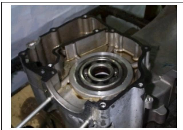
Scrape gasket residues off the crankcase contact surface.
