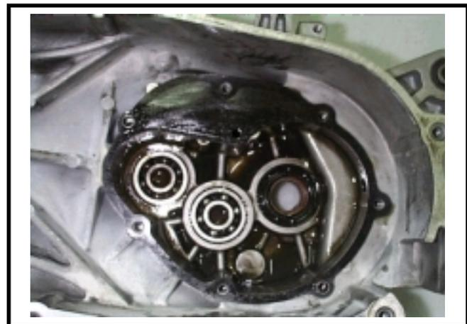
Remove oil seal, and then remove final shaft bearing from left crankcase.
