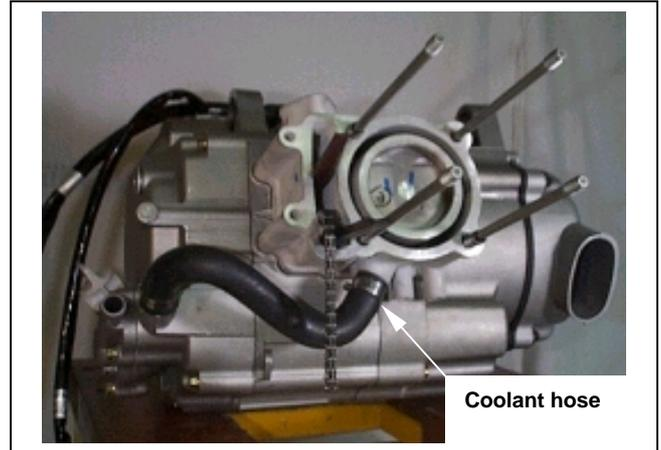
Remove cylinder gasket and dowel pin.
