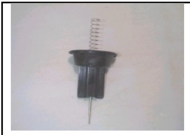
Remove compress spring and vacuum piston.
