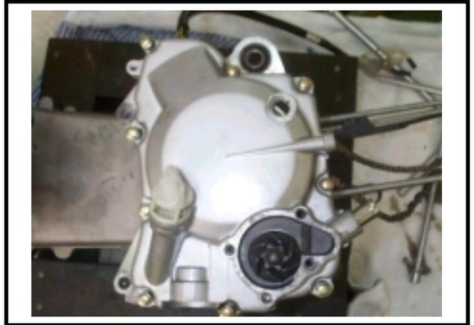
Turn pump rotor clockwise and remove.
