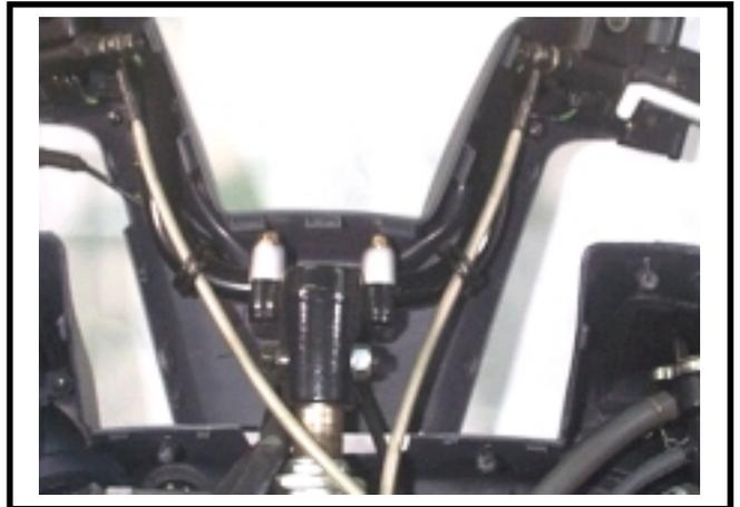
Remove the right switch assembly by loosening two screws.
