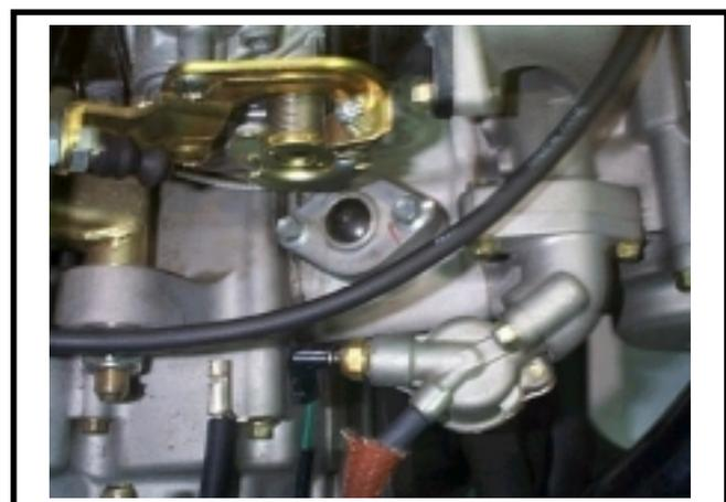
Removing the reserve tank filler cap.
