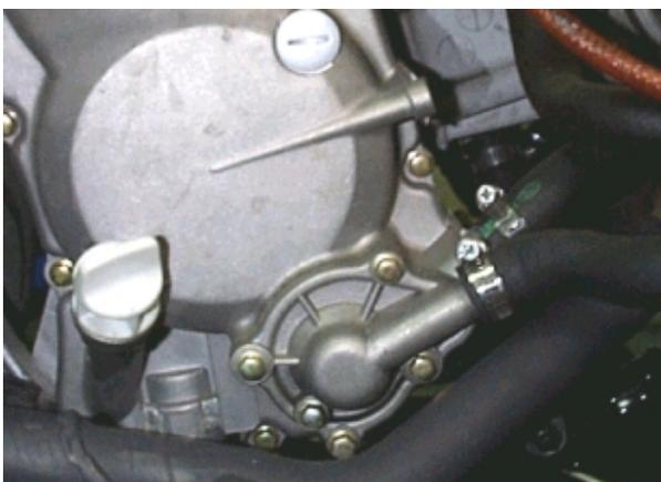
Loosen 2 nuts and 4 screws.
