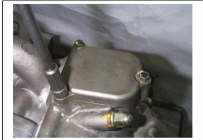
Remove the rocker arm pin stopper plate, and then screw a 5mm bolt into the rocker arm pin. Finally, remove the pin and the rocker arm.
