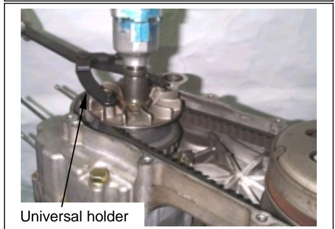
Tighten nut to specified torque.
