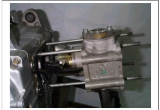
Install coolant hose onto cylinder.
