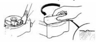
The ends of rubber hoses (for fuel, vacuum, or coolant) should be pushed as far as they can go to their connections so that there is enough room below the enlarged ends for tightening the clamps.
