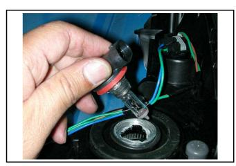
Turn the position light set and then remove the position light bulb seat.
