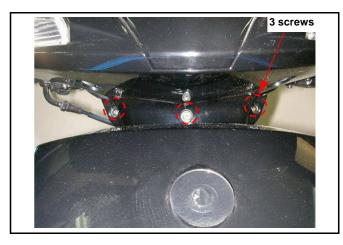
Remove front winker light electric cord couplers. Remove handle front cover.
