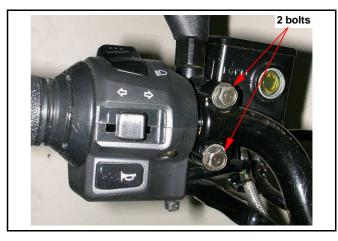
Remove left handle switch after left handle switch mounting screws removed. (2 screws)
