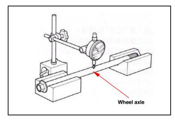
Place the wheel on to a rotation seat, and turn the wheel to check its bearing free play. If the bearing is noisy or its free play is too much, replace it.
