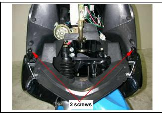
Pull up the front inner spoiler from holder hook, and then remove the front inner spoiler and right / left under spoiler assembly.
