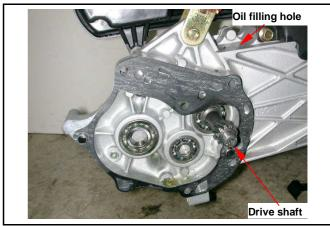
Drive shaft is pulled out with it's bearing, then remove the bearing with bearing puller and shaft protector.
