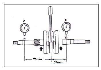
Check the crankshaft bearing by means of turning it with hand. If any noise and bigger clearance are detected, replace the bearing with new one.
