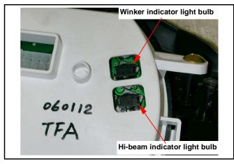
Replace with new bulb if necessary.
