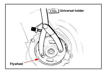
Tighten nut to specified torque. **Torque value:** 5.5~6.5kgf-m Install left crankcase cover.
