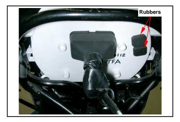
Turn the bulb seat in counter-clockwise direction and then remove, and then take out the bulb seat from the bottom of instrument panel.
