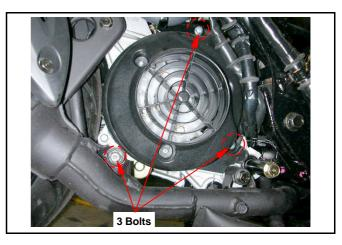
Remove 4 bolts, and then take out the cooling fan.
