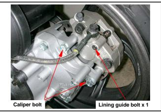
Remove the brake pad guide pin bolt and locking spring, and then remove brake pads.
