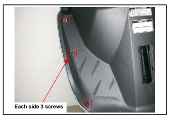
Remove 2 screws from the front upper part of the front spoiler and the front inner box.
