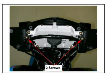
Remove speedometer electric cord coupler. Remove handle rear cover.
