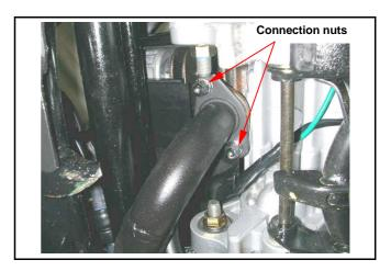
Remove exhaust muffler bolt (3 bolts), then remove the muffler.
