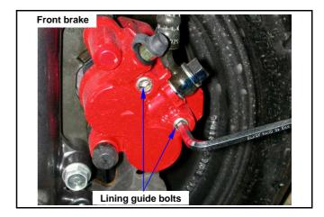
Remove brake caliper mounting bolt and then remove the brake caliper.
