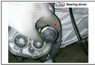
Install new bearings into gearbox cover.
