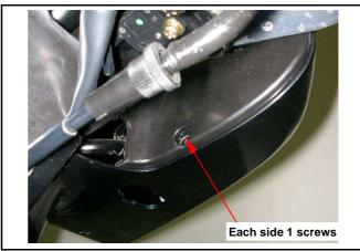
Remove 3 screws from the handle front cover under.
