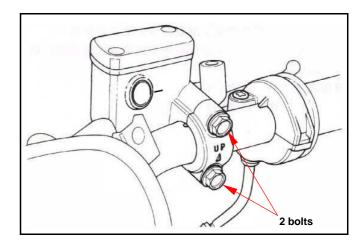
Install the brake lever, and connect leads to brake light switch.
