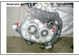
Install counter shaft, counter shaft side washer and final shaft into the gearbox.
