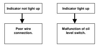
5. Disconnect oil level switch coupler, and check voltage between wire and ground.
