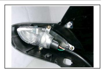
Push and turn the bulb in counter-clockwise direction, and then remove the bulb. Replace with new bulb if necessary. **Specification:**
