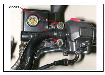
Remove throttle grip and right handle switch after right handle switch mounting screws removed. (2 screws)
