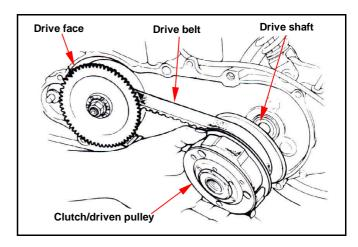
Hold the clutch outer, and then tighten nut to specified torque value.
