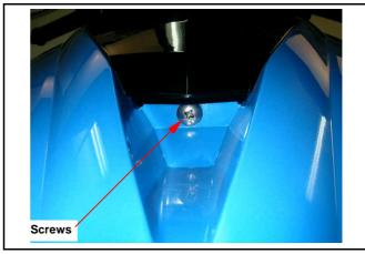
Remove electric cord coupler from the headlight. Remove the front cover.
