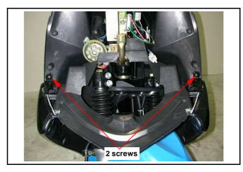
Remove 6 screws from the front inner box and under spoiler.
