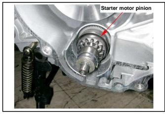
Check the pinion for sliding in axial direction smoothly.
