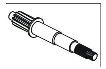
Check if the countershaft is wear or damage and replace it if necessary.
