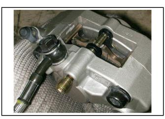
Install the new brake pads onto brake caliper.
