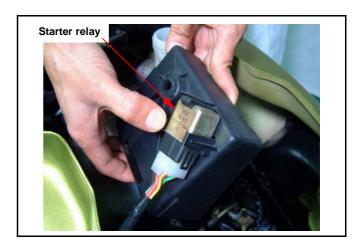
Connect both the green/yellow (-) and the yellow/red (+) pins to battery posts directly. If the red and red/white pins are also in continuity, it means it is in normal.
