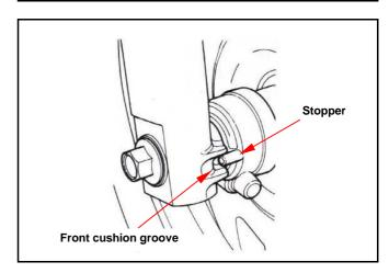
Insert the wheel axle into the wheel, and then install the wheel axle nut.
