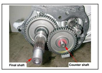
Remove the drive shaft from left crankcase.
