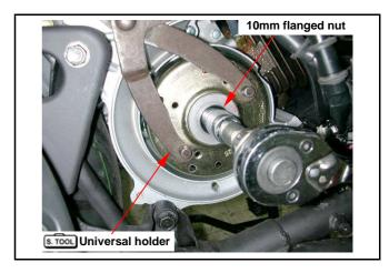
Remove the flywheel with flywheel puller.
