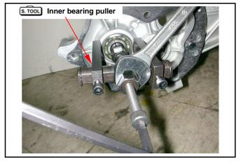
Install new bearings into left crankcase.
