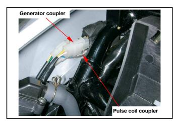
Remove the pulse coil and generator coil bolts (4 bolts), and then take out the generator assembly.
