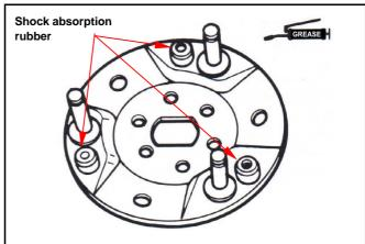
Install new clutch weight onto lock pin and then push to specific location.
