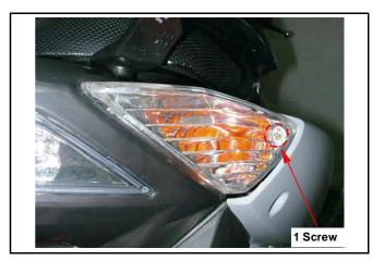
Remove rear winker inner lens. (1 screw)
