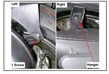
Ramoval rear mudguard right side bolt, and then remove rear wheel.
