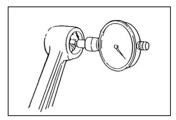
Install bearing and piston pin onto connecting rod small end, and then check its clearance.
