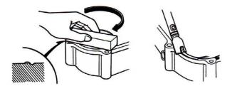
The ends of rubber hoses (for fuel, vacuum, or coolant) should be pushed as far as they can go to their connections so that there is enough room below the enlarged ends for tightening the clamps.
