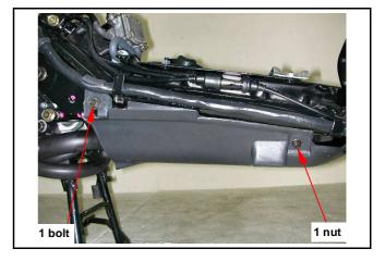
Remove 1 bolt and 1 nut from the under cover left side, and then remove under cover.
