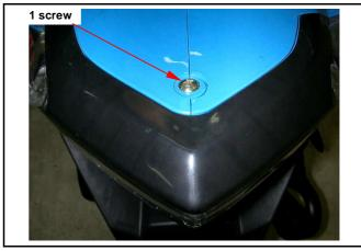
Remove 4 screws and then remove taillight assembly.
