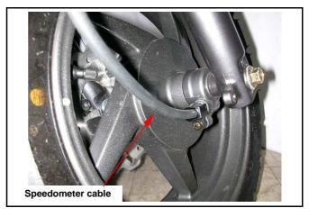
Remove front wheel axle nut, and then pull out the axle and remove the wheel.
