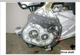
Drive shaft is pulled out with it's bearing, then remove the bearing with bearing puller and shaft protector.
