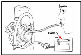
Check resistor to make sure that the auto by-starter is in normal. Engine is running. If the resistor is in open-circuit, then current will not flow into the PTC. Thus, the auto by-starter is not operated.
