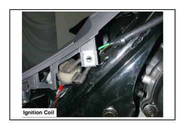
Measure the primary coil resistance. Resistance:  $0.19 \sim 0.23 \Omega$  (A) $\rightarrow$ (B) Measure the secondary coil resistance. Resistance:  $8.2 \sim 9.3 K\Omega$  (A) $\rightarrow$ (D)
