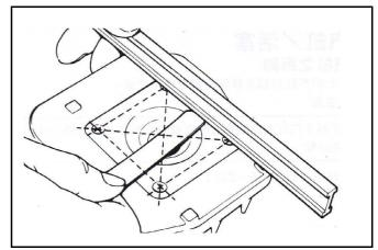
In "X" and "Y" direction, measure the cylinder for worn out as the three levels shown in the figure. With the maximal value to decide cylinder wear out condition.
