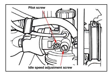
Adjust the idling after warn up engine for 10 minutes.
