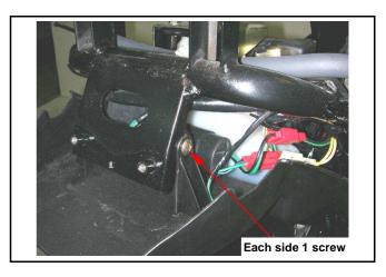
Pull out rear fender front hanger with frame, and then removal rear inner fender.
