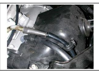
Remove fan cover (3 bolts). Remove engine shield mounting bolt (1 bolt).
