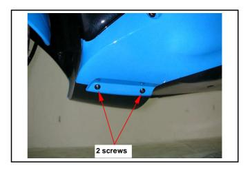
Remove 2 screws, and then slide the side cover backward so that their hooks are out of slots. Take out the side cover end part and then remove the cover.
