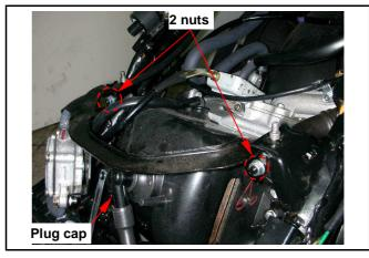
Remove vacuum tube and oil pump control cable from engine shield.
