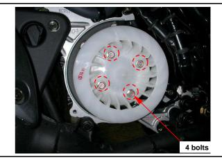
Hold flywheel with universal holder. Support the flywheel and the remove the 10 mm nut on the flywheel.
