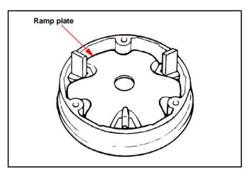
Apply with some grease to inside of movable drive face, and install drive face boss.
