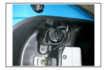
Remove luggage box mounting nuts and bolt (2 nuts & 1 bolt).
