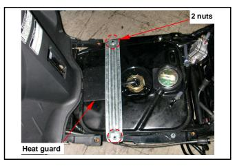
Disconnect fuel unit coupler from front wheel side.
