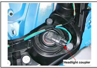
Turn the set in counter-clockwise direction, and then remove the bulb.
