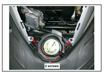
Remove 2 screws from right / left center cover and floor panel other side.
