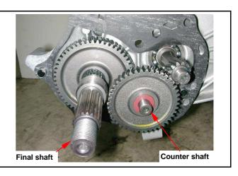
Remove the drive shaft from left crankcase.
