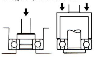
Both of these examples can result in bearing damage.
