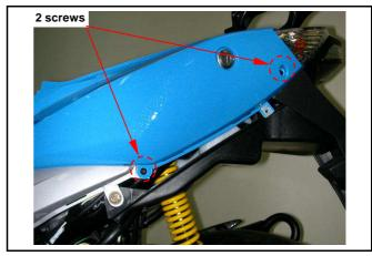
Remove 2 bolts from the rear fender. Slide the body covers and taillight backward so that their hooks are out of slots. Take out the body covers and taillight end part and
