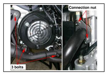
Support the engine and then remove cushion lower mounting bolt.
