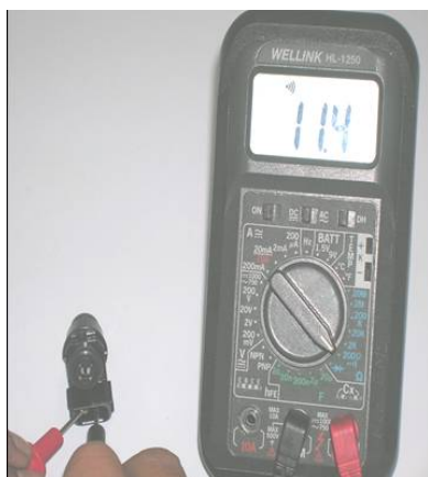
Injector resistance confirmation
