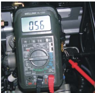
Throttle output signal measurement - full closed
