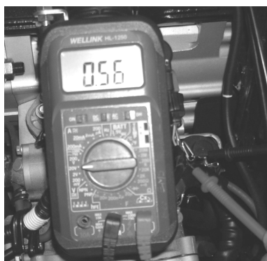
Throttle output signal measurement - full closed
