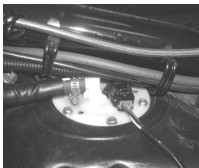
Fuel pressure measurement demolition - fuel pump
