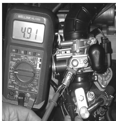
Working voltage measurement
