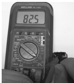
B phase measurement of the resistance value
