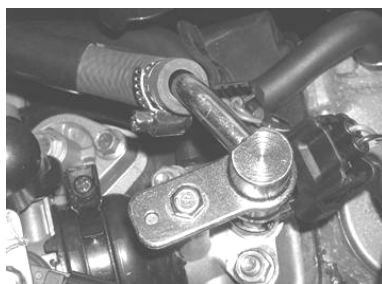
Fuel pressure measurement demolition - injector
