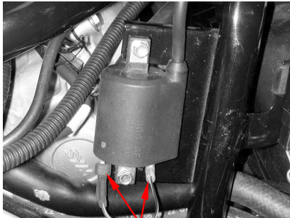
First circuit coil resistance measurement
