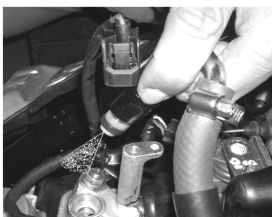
Injection-state atomizing good
