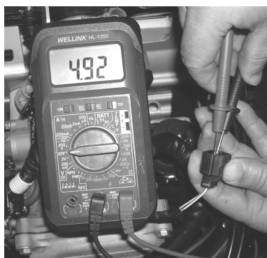
Working voltage measurement
