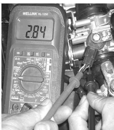
Output voltage measurement plains
