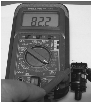
A phase measurement of the resistance value
