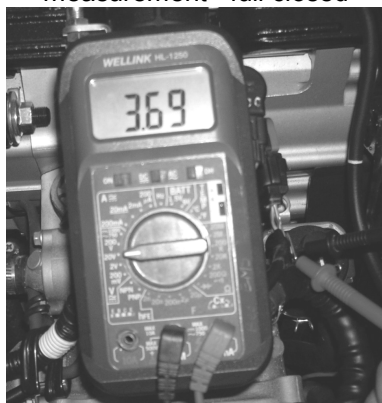
Throttle output signal measurement - full
