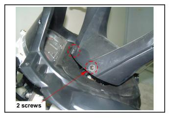
Loosen the 2 screws from handle upper cover rear end.
