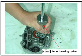
Remove oil seal, and then remove final shaft bearing from gear box cover using following tools. **Special tool:**
