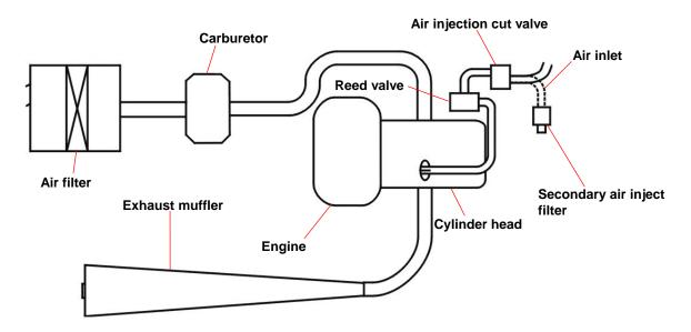
• If no sound is heard, remove air cut-off valve, and connect a vacuum meter to air pipe to check for leakage.
