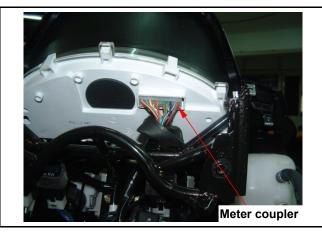
Loosen 4 screws from meter panel. Remove the speedometer.
