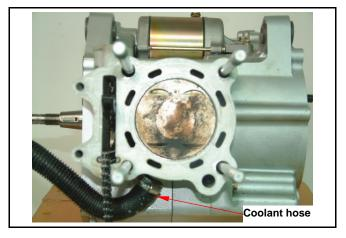
Cover the holes of crankcase and cam chain with a piece of cloth.
