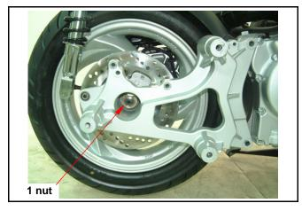
Remove rear fork and both side collars. Remove the rear wheel.
