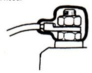
If fuse burned, it has to find out the cause and solved it. And then replace with specified capacity fuse.
