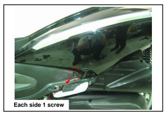
Loosen right and left side screws from rear side of the body cover.
