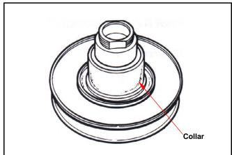
Remove guide pin, guide pin roller, and movable driven face, and then remove O-ring & oil seal seat from movable driven face.
