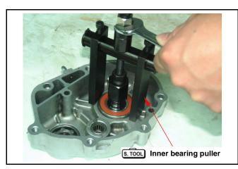
Install a new drive shaft bearing and counter shaft bearing into gear box cover.
