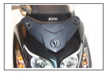
Disconnect the coupler of the speedometer, and take off the meter panel and meter.
