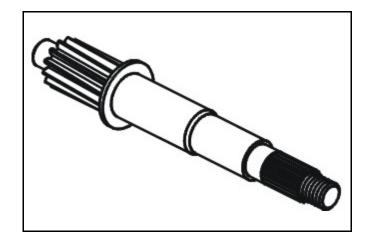
Check if the countershaft is wear or damage and replace it if necessary.
