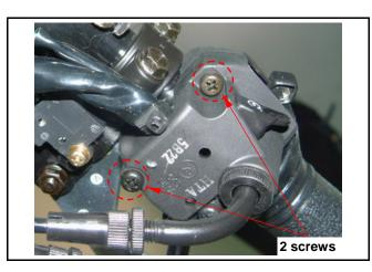
Remove throttle holder, handle switch, cables and grip.
