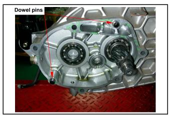
Install counter shaft and final shaft into the gear box cover.
