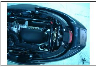
Remove right and left side covers (4 screws on each side.).
