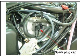
Loosen 2 bolts and replace the ignition coil if necessary.
