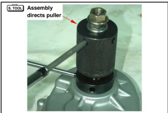
Apply with grease onto final shaft oil seal. Install the oil seal into gear box cover.
