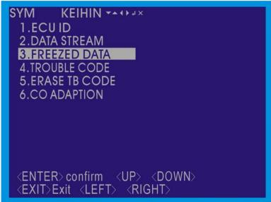
Only one page, at any screen, press the "EXIT" button, the function can return to the directory screen. In the "FREEZED DATA" of the screen use "▲" "▼" button to move the left side of the project "→" symbol selected items, press the "ENTER" buttom lock of the project, and press the "F4" button showed that the wave of projects.
