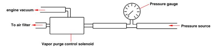
2) Apply 100mmAq into pressure source inlet as engine stopped then plug it. The pressure at the gauge should not drop to below 10mmAq within 10 seconds.
