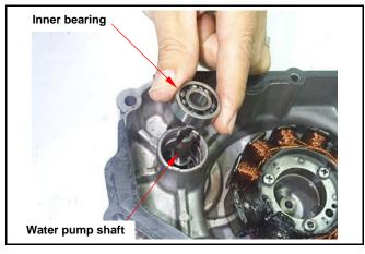
Install the cir clip to hold the inner bearing.
