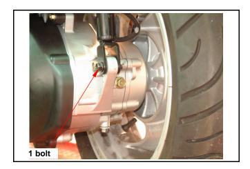
With a bracket to support the engine to prevent from it damage by falling down as removing the engine.
