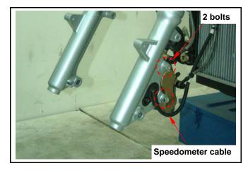
Loosen 4 bolts from steering stem. Remove the front cushions.
