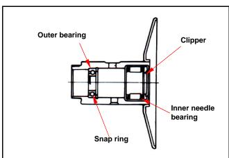
Remove snap ring and then push bearing forward to other side of inner bearing.
