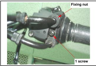
Loosen 2 screws from the throttle holder.
