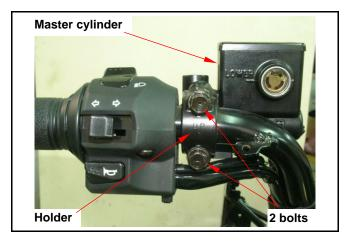
Loosen left handle switch connecter. Loosen 2 screws from left side handle switch holder.
