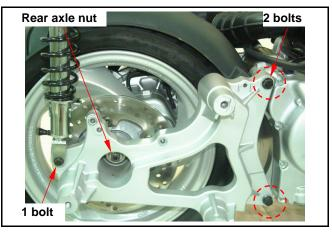
Remove the rear fork and rear axle collars.
