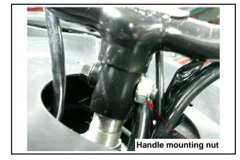
Apply with grease onto throttle cable and the sliding surface of handle.
