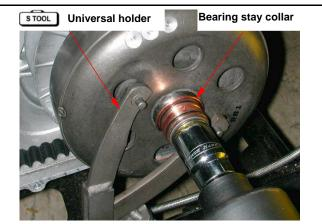
Push the drive belt into belt groove as diagram shown so that the belt can be loosened, and then remove the driven pulley.
