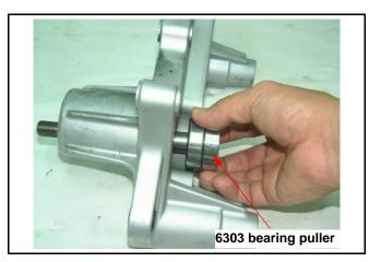
Install the washer of the 6303 bearing puller.
