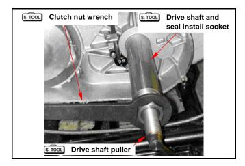
Apply with grease onto drive shaft oil seal. Install the oil seal to left crankcase.
