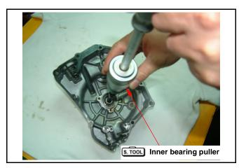
Install the bearing 6201 bearing with special tool. **Special tool:**
