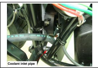
Loosen the cooling fun mounting bolts (3 bolts). Remove thermo switch.
