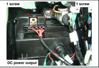
Loosen 1 screw from battery cover and remove it.
