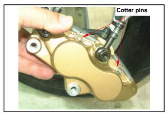
Remove the brake pad shafts and pads.
