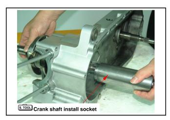
Turn in the crank shaft puller spiral tooth to the left crank shaft.
