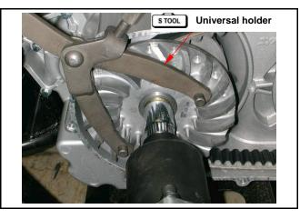
Hold clutch outer with universal holder, and remove nut, bearing stay collar and clutch outer.
