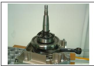
Install 2 dowel pins and new gasket.
