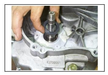
Install the oil seal in the left crankcase with special tool.
