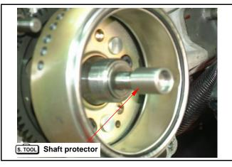
Remove starter reduction gear and shaft. Pull out flywheel with AC.G. flywheel puller. Special tool:
