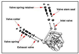
Put the valve cotters onto valve spring retainer. Use a valve cotter remove & assembly tool to press the valve springs, and then install valves.
