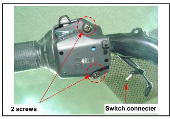
Loosen handle mounting nut. Remove handle mounting bolt, and then remove the handle.
