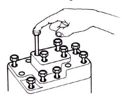
Tighten assemblies with different dimension fasteners as follows: Tighten all the fasteners with fingers, then tighten the big ones with special tool first diagonally from inside toward outside, important components should be tightened 2 to 3 times with appropriate increments to avoid warp unless otherwise indicated. Bolts and fasteners should be kept clean and dry. Do not apply oil to the threads.
