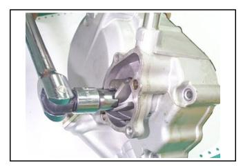
Remove the cir clip from the right crankcase cover. Remove the water pump shaft and the inner bearing.
