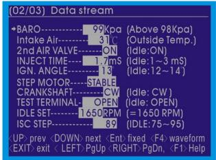
The screen showed the ECU captured by the engine of the state immediately. The following data for the benchmark idling state:
