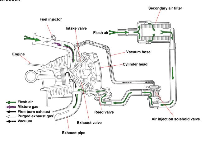
This system contained AISV (air Injection Solenoid Valve), Reed Valve and other intake components.
