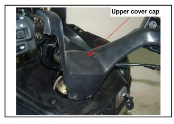
Loosen the 3 screws from the handle upper cover, and then remove handle upper cover.
