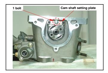
Remove rocker arm shafts and rocker arms. **Special Service Tool:** Rocker arm and cam shaft puller SYM-1445100
