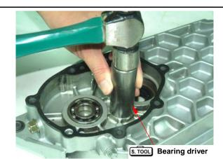
Install new drive shaft bearing and bearing puller onto left crankcase.
