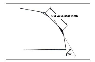
Use 45° cutter to grind the valve seat to specified width.
