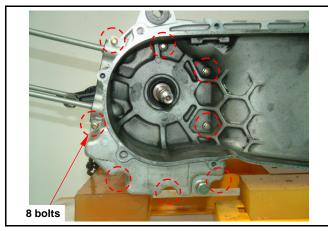
Place right crankcase downward and left crankcase upward.
