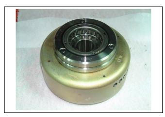
Install start clutch driven gear onto one way clutch. Hold flywheel and rotate start clutch gear. The start clutch gear should be rotated in C.C.W direction freely, but not C.W direction. (View as shown in this figure.)
