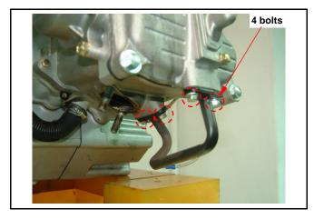
Remove the cylinder head side cover.
