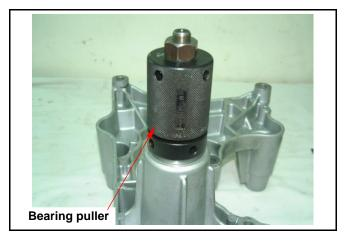
Use screw driver holder bearing puller lower part, and turn the bearing puller upper part to install the rear fork bearing.
