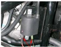
First circuit coil resistance measurement
