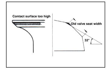
If the contact surface too high, grind the valve seat with 32° cutter.
