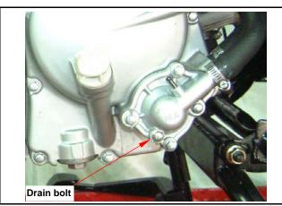
Refilling system with coolant and bleeding the air bubbles.
