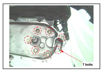
Remove the gear box cover. Remove the gasket & dowel pin.
