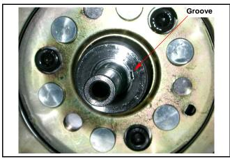
Hold the flywheel by drive face with universal holder, and tighten flywheel nut. Torque value: 5.0~6.0kgf-m
