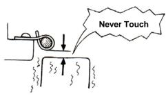
Route wire harnesses to avoid sharp edges or corners and also avoid the projected ends of bolts and screws.
