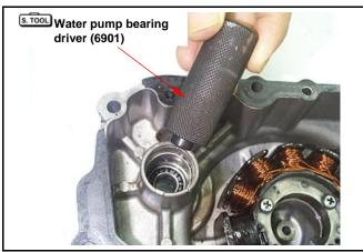
Mount the water pump shaft and the inner bearing to the right crankcase cover.
