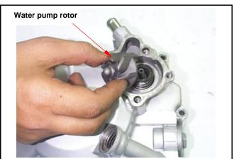
Install the dowel pin and right cover gasket. The rotation water pump rotor, causes the water pump drive shaft scoop channel, aligns the oil pump drive shaft flange, install the right crank case. (10 bolts)
