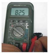
B phase measurement of the resistance value
