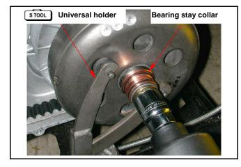
Install the drive face, washer and drive face nut. Hold drive face with universal holder, and then tighten nut to specified torque value.
