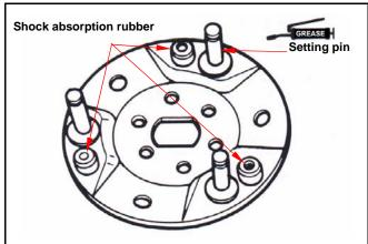
Install new clutch weight onto setting pin and then push to the specified location.
