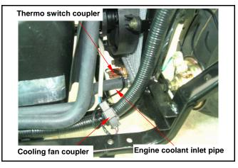
Remove reserve tank coolant inlet pipe. Remove the radiator and the cooling fun.
