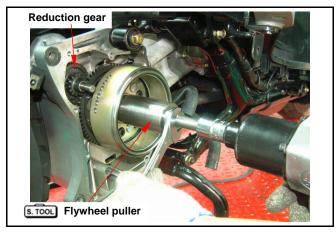
Remove flywheel and starting driven gear.
