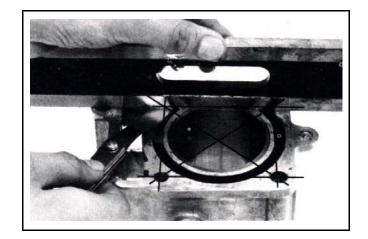
Measure the clearance between piston rings and ring grooves.
