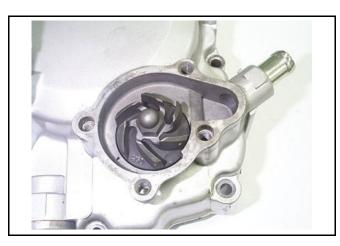
Install the dowel pin and new gasket. Install the water pump cover with 4 bolts.
