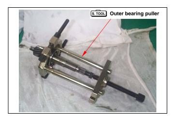
Remove final shaft bearing and counter shaft bearing from left crankcase using following tools. **Special tool:**
