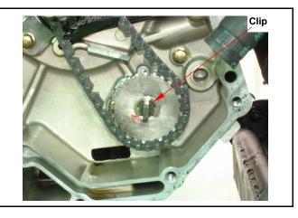
Install starting gear and generator. (Refer to chapter 10)
