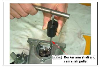
Remove cam shafts. Special Service Tool: Rocker arm and cam shaft puller SYM-1445100
