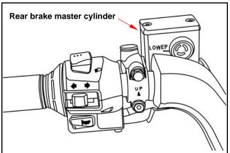
Remove the master cylinder cap and diaphragm. Increases the high quality brake fluid, uses by all means must with the trade mark brake fluid joins in the master cylinder.
