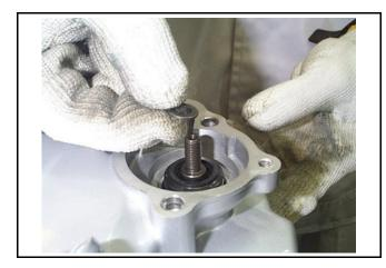
Install the rotor onto the water pump shaft and tighten.
