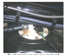
Fuel pressure measurement demolition - fuel pump
