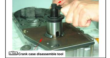
Install crank shaft onto the left crankcase and install crank shaft install socket.
