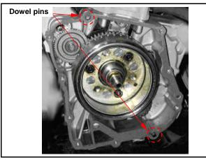
Install right crankcase cover (10 screws). Install the dowel pin, new gasket and water pump cover onto crankcase cover.
