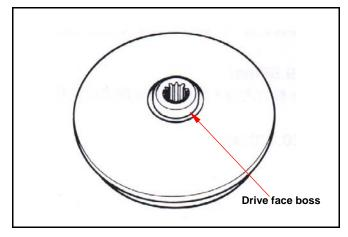
Install movable drive face comp. onto crankshaft.
