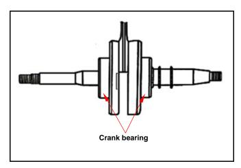
If any roughness, noise and loose linkage are detected, replace the bearing with new one.
