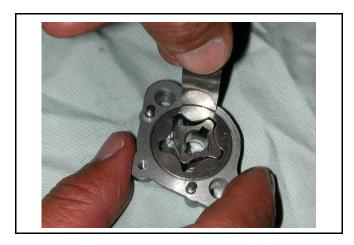
Check clearance between inner and outer rotors.
