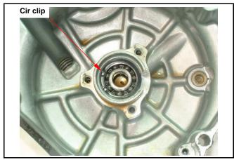
Remove the bearing 6201with inner bearing puller. **Special tool:**
