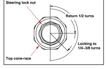
Install the steering stem mounting nut and tighten the nut by means of holding the top cone race body.
