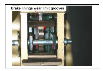
The brake pad must be replaced with new lining when the brake pad wear limit reaches the brake disk.
