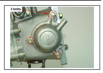
Remove left crankcase cover, and turn the Turn the drive face, and align the timing mark on the sprocket with that of cylinder head, piston is at TDC position.
