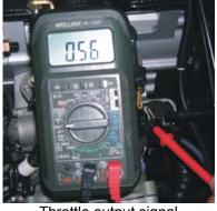
Throttle output signal measurement - full closed
