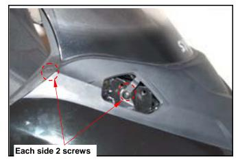
Loosen 6 screws from the wind screen and remove the wind screen.
