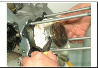
Remove cylinder gasket and dowel pin.
