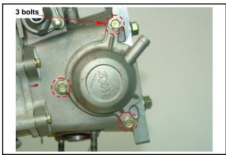
Remove left crankcase cover, and turn the drive face, and align the timing mark on the cam sprocket with that of cylinder head, piston is at TDC position.
