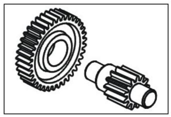
Check if the final shaft and gear are burn, wear or damage and replace it if necessary.
