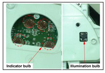
Uses the slotted screwdriver to turn the indicator bulb seat in C.C.W. direction, and remove the indicator bulb.
