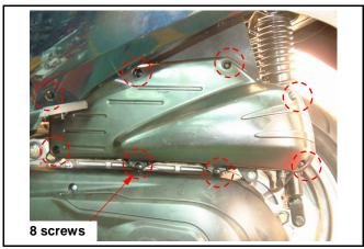
Remove the body cover. Loosen bolt from the air cleaner air hose.
