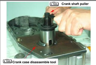
Remove crankshaft and wave washer from right crankcase.
