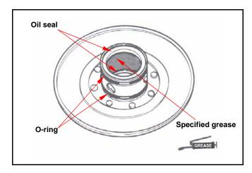
Install the movable driven face onto driven face. Install the guide pin and guide pin roller.
