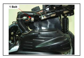
Remove the air cleaner connection bolts (2 bolts). Remove the air cleaner.
