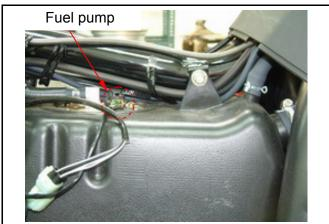
Remove the fuel tank fixed bolts (Bolt × 3), remove the fuel tank.
