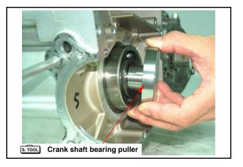
S. TOOL Crank shaft puller
