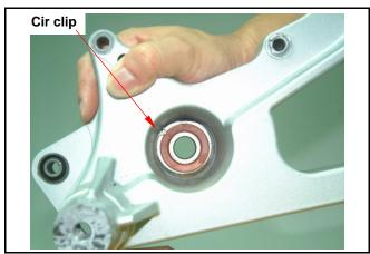
Uses the bearing driver; drive out the bearing.
