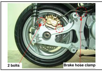
Remove the right rear cushion lower bolt (1 bolt). Remove the rear fork bolts (2 bolts). Remove the rear wheel axle nut (1 nut).
