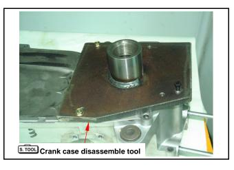
Install left crank shaft puller into crank case disassemble.
