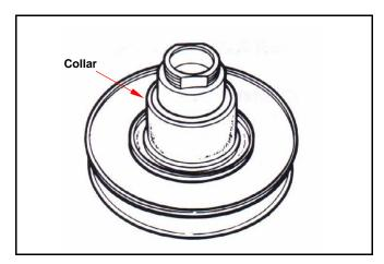
Install friction plate, spring and clutch weight into clutch spring compressor, and press down the assembly by turning manual lever until mounting nut that can be installed.
