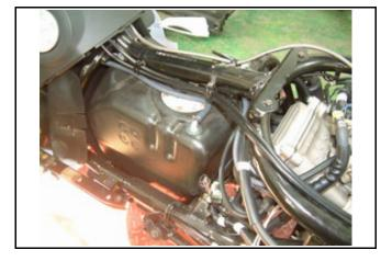
Remove fuel pump lines coupler. Release the fuel tube folder, removed the fuel tube.
