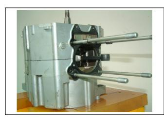
Tighten 8 bolts on the left crankcase. Tighten 2 bolts on the left crankcase.
