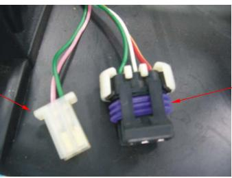
Diagnostic tool coupler and test switch coupler plant
