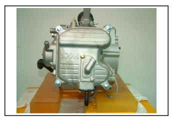
Remove 2 bolts of thermostat and then remove the thermostat.
