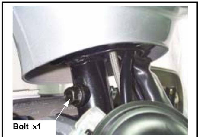
Remove the handlebar assembly.
