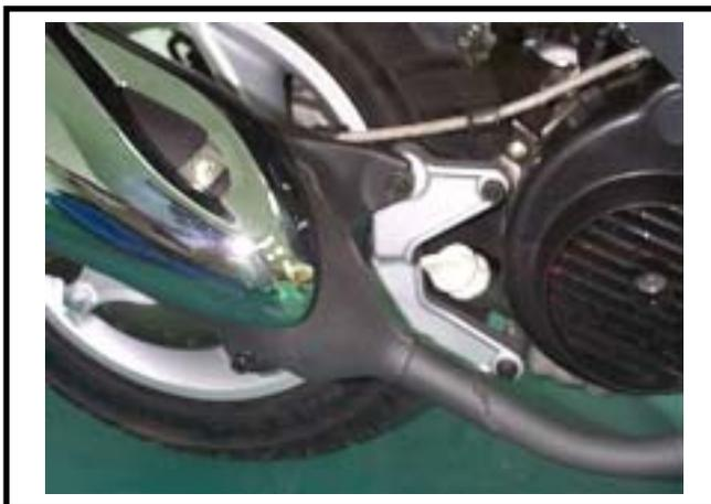
Remove the cooling fan. (4 bolts)
