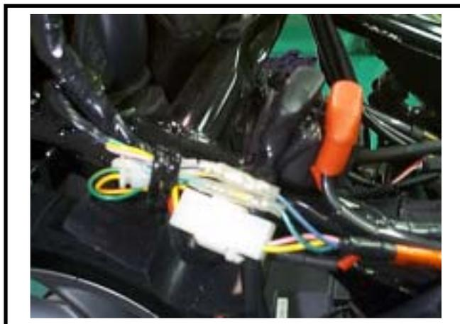
Remove the starter motor cable on the relay.
