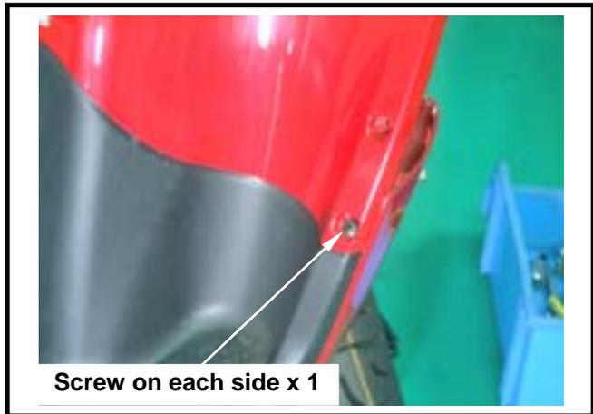
Remove 2 screws on the left & right each side of side cover.
