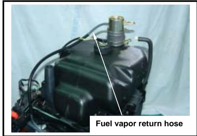
Remove the fuel hose and then remove the fuel tank.
