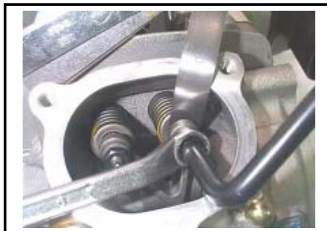
Start the engine after assembly. Remove the intake valve adjustment hole cap and make sure that engine oil flows onto the cylinder head. Stop the engine after confirmed, and then install the intake valve adjustment hole cap. Install the seat cushion and the central cover.
