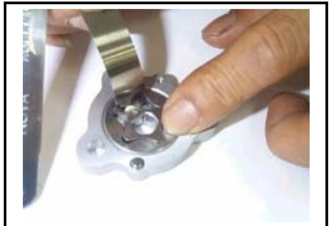
Check clearance between rotor side face and pump body.
