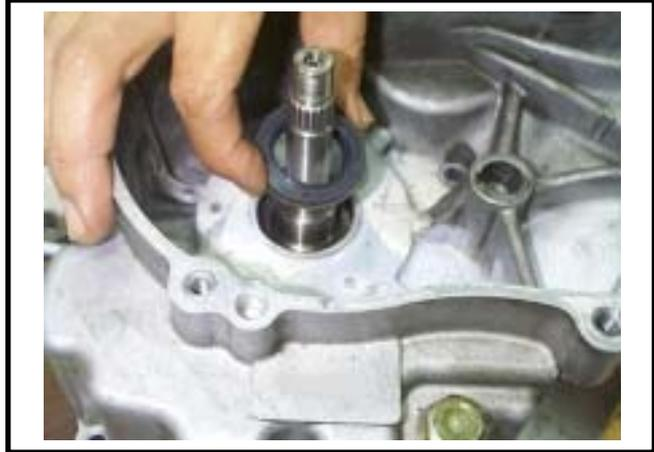
Press-fit the oil seal to specified position with the oil seal installer (25x37x6).
