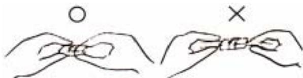
Make sure if the connector pins are bent, extruded or loosen.
