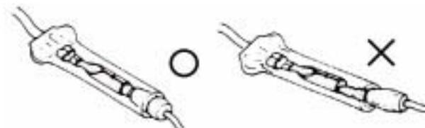
Secure wires and wire harnesses to the frame with respective wire bands at the designated locations. Tighten the bands so that only the insulated surfaces contact the wires or wire harnesses.
