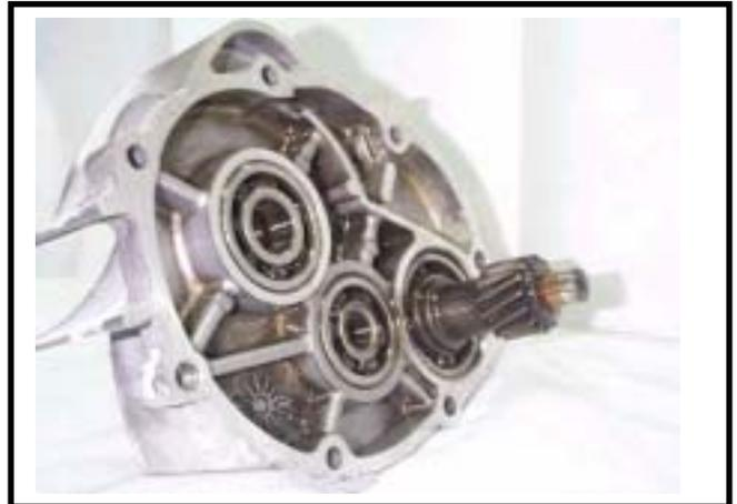
Install a new final driving shaft bearing onto gear box cover.
