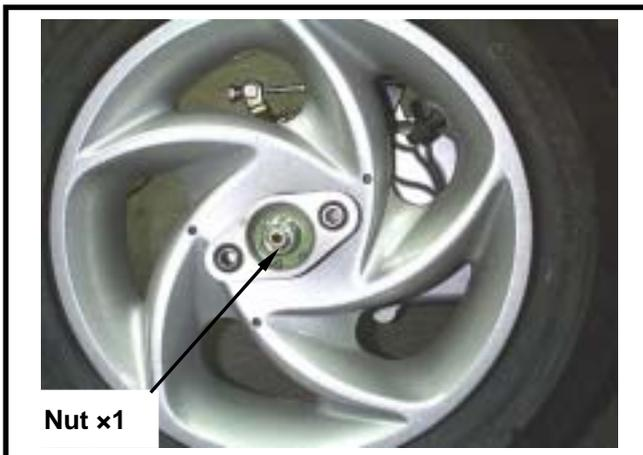
Remove the rear brake adjustment nut.
