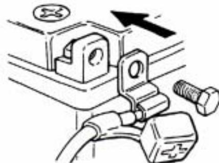
Make sure that the battery post caps are located in properly after the battery posts had been serviced.
