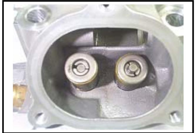
With the valve spring remover/installer, compress the valve spring directly. Then, remove the valve and valve spring.
