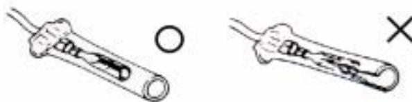
Insert the terminal completely. Check if the terminal is covered by the boot. Do not let boot open facing up.
