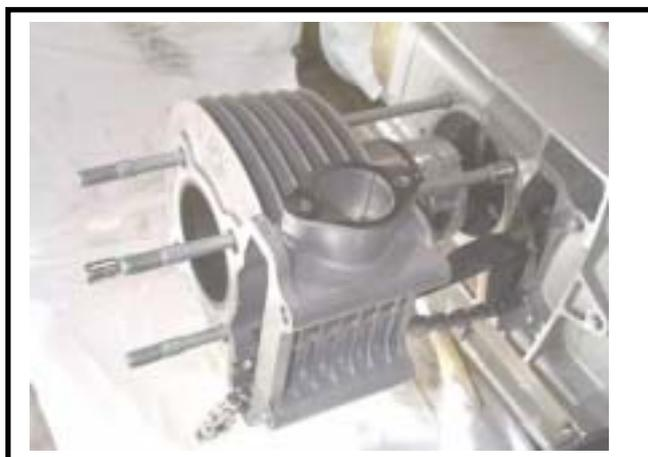
Install the cam chain plate, the cylinder gasket and lock pins.
