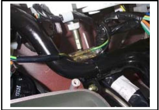
Remove the winker relay coupler.
