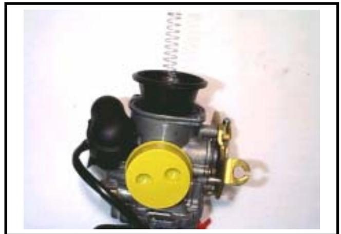
Install vacuum chamber cover and tighten 2 screws.
