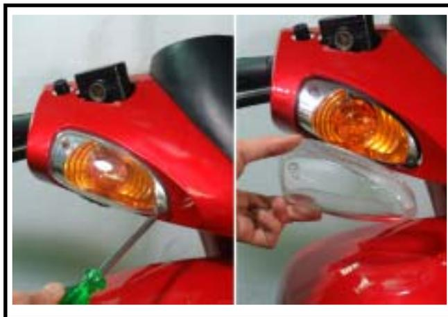
Remove the light inner cover of the turn signal lamp. (screw x 1)
