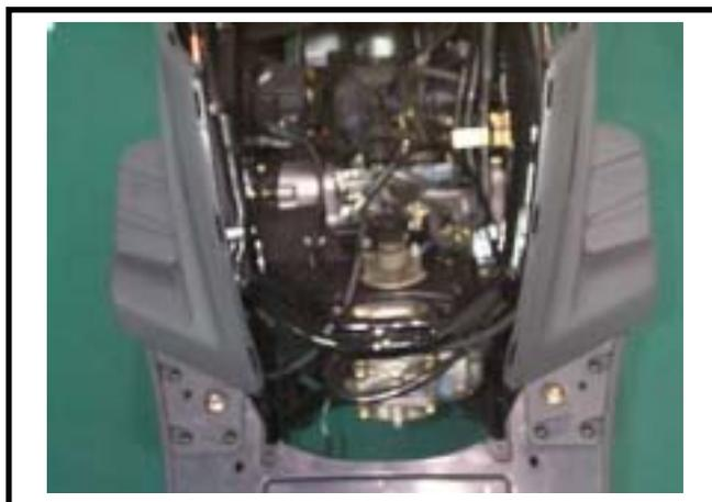
Remove the connector of rear lamp power wire and generator wire.
