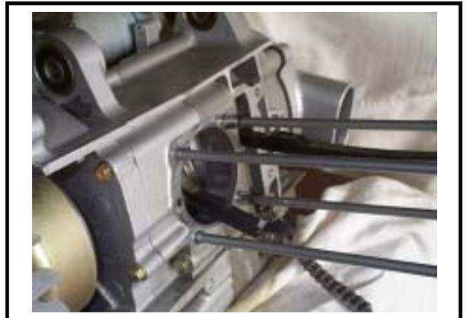
Clean the residues attached onto the matching surfaces of cylinder and crankcase.
