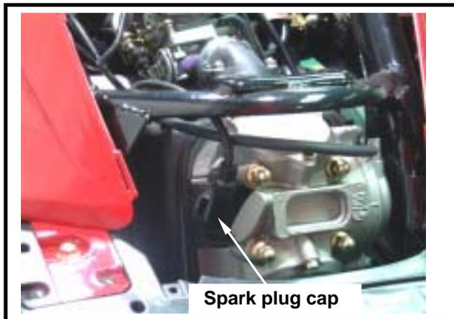
Loose the throttle valve cable fixed nut and remove the throttle valve cable.
