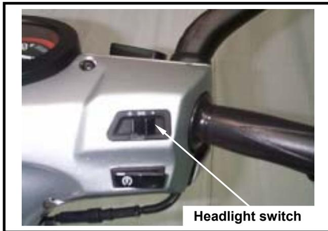
**High/Low beam switch & Passing switch**
