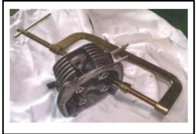
Or with the valve spring remover/installer to install valve and spring.
