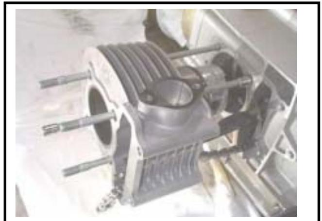
Remove cylinder gasket and lock pins.
