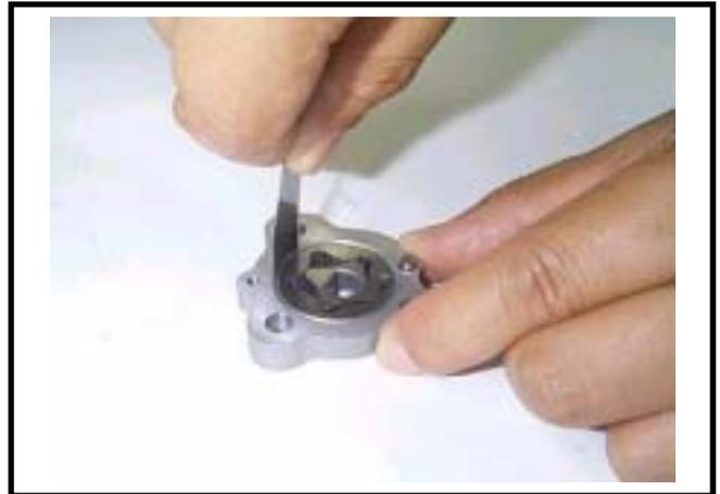
Check clearance between inner and outer rotors.
