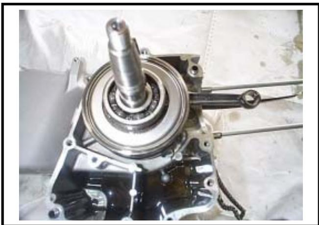
Remove oil seal from the left crankcase side.
