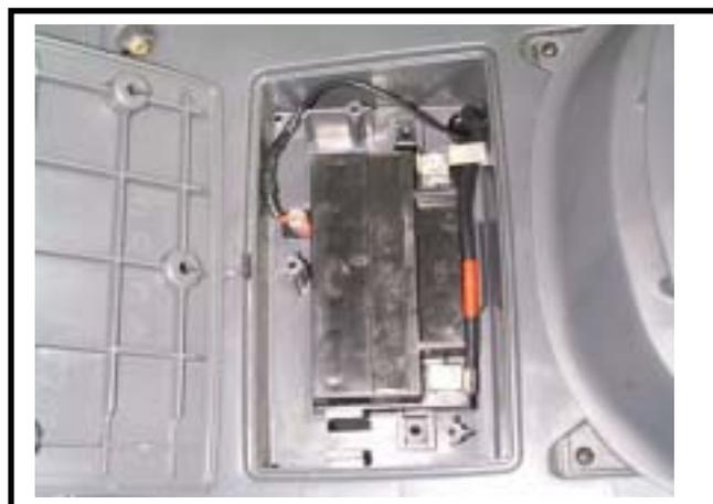
Remove the bottom mounting screws from the floor panel, and then the floor panel.
