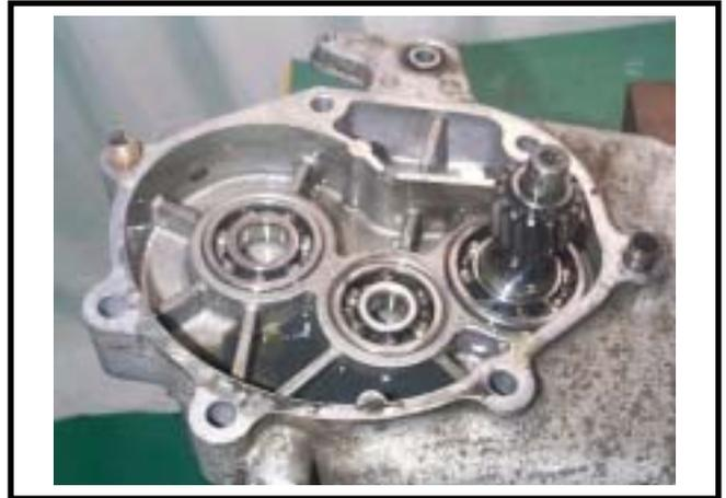
If the driving shaft is pulled out with its bearing, then remove the bearing with bearing puller and bearing protector.
