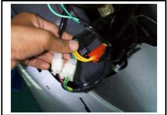
Remove the rear cover of the handlebar. (chapter 12, section 3)
