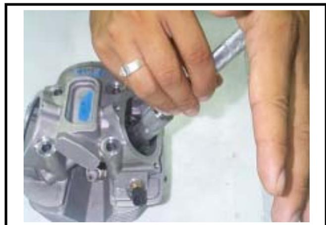
Special Service Tool: Valve spring remover/installer.
