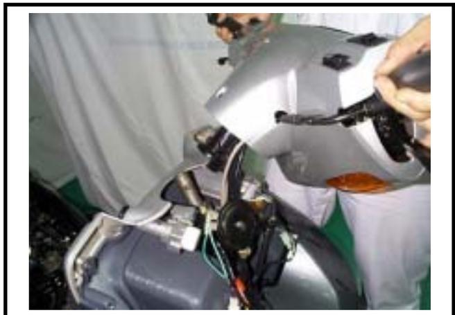
Remove the main switch connector and bolts. (bolts x 3)
