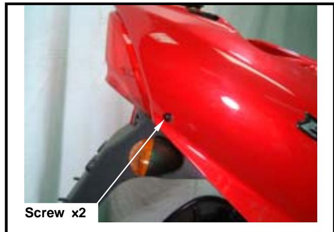
Remove the seat lock cable, then remove the body cover.
