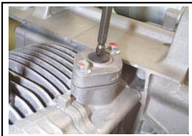
Remove the cam sprocket. (bolt x2)
