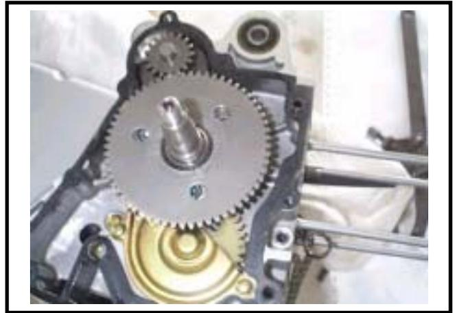
Remove starting clutch, starting idle-gear, and shaft.
