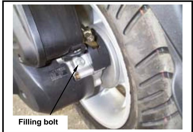
Remove gear oil filling hole bolt and place a measurement cup under the draining plug. Remove the oil draining plug and the pour gear oil into the measurement cup. Measure the gear oil quantity if within standard value. Add specified gear oil if the oil level too low. (Standard quantity: 110cc. / replacement: 100 cc.)
