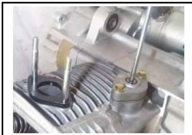
Install the left-side cover of the engine body. (bolt x 1)
