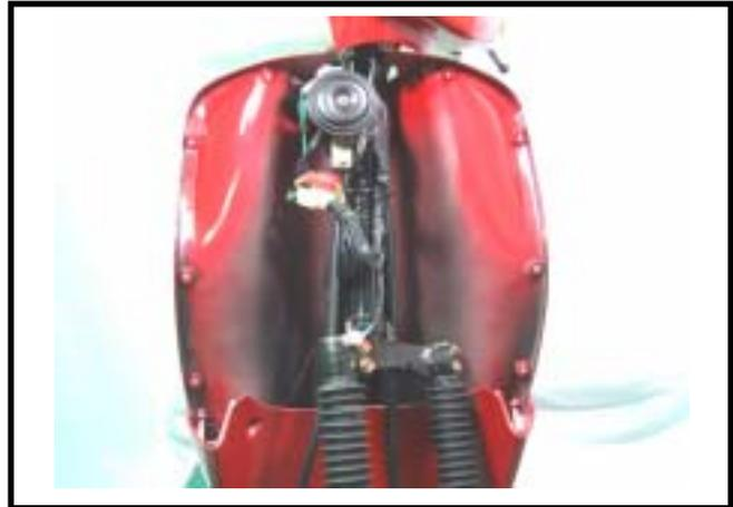
Remove the power coupler of the meter.
