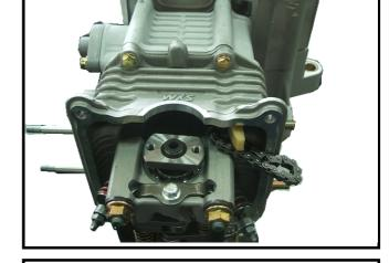
Remove the 2 cylinder head mounting bolts from cylinder head left side cover.
