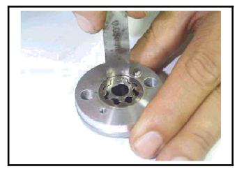
Check clearance between inner and outer rotors.
