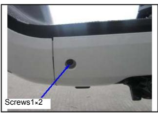
Remove the 6 mounting screws between the front cover and the front inner box.
