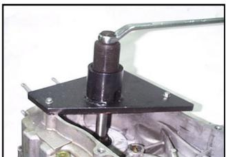
Remove the crankshaft from the right crankcase.
