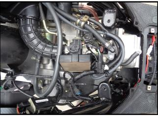
Remove the fuel tube. Remove cylinder head TEMP sensor connector.
