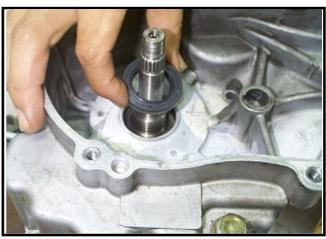
Press-fit the oil seal to specified position with the oil seal installer (19.8x30x5).
