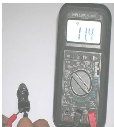
Injector resistance confirmation
