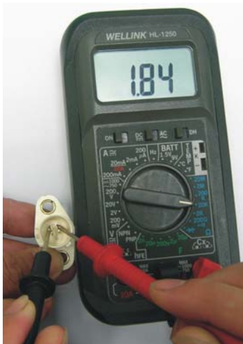
Resistance value measurement
